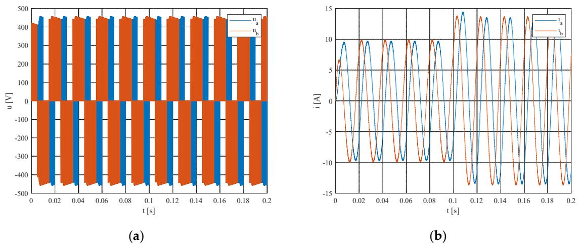
**Figure 24.** VSI inverter voltages (a) and currents (b) in  $a, b$ , resp. in  $\alpha, \beta$ - systems during the transient.
