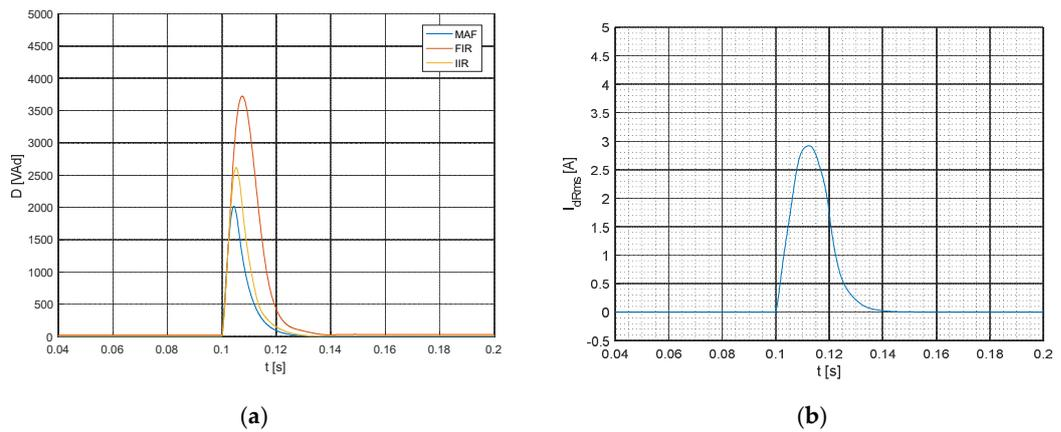
**Figure 12.** Waveforms of distortion power components  $D_{av}(k)$  during transient states calculated by different methods (MAF-, DFIR, and DIIR filters) (a), and the corresponding deformation component of the current using the MAF method (b).
