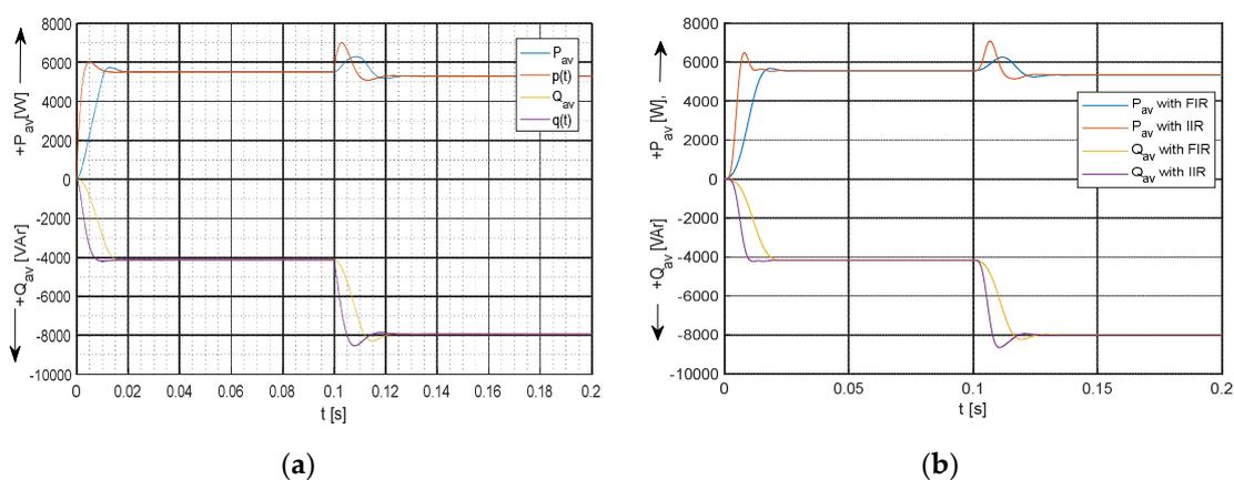
Figure 4. Comparison of power waveforms calculated by different methods MAF and direct function in the time domain  $p(t)$  and  $q(t)$ —(a), DFIR and DIIR filters for  $P_{av}(k)$  and  $Q_{av}(k)$ —(b).
