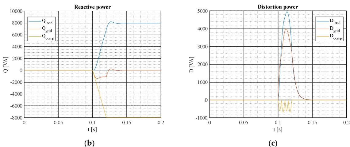
**Figure 31.** Using switched capacitors (a) for compensating reactive blind power (b) under linear RL load and distortion power (c).
