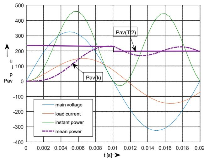
**Figure 1.** Principal time-waveform of  $P_{av}(k)$  by using of MAF method: step  $k = 0.5 \text{ ms}$ , length of sliding window  $l = T/2 = 0.01 \text{ s}$ .
