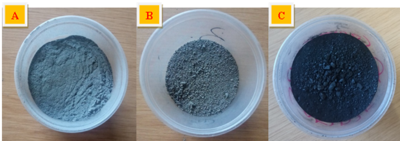
Figure 1. (A) Bituminous coal fly ash, (B) bottom ash, and (C) raw coal samples.
