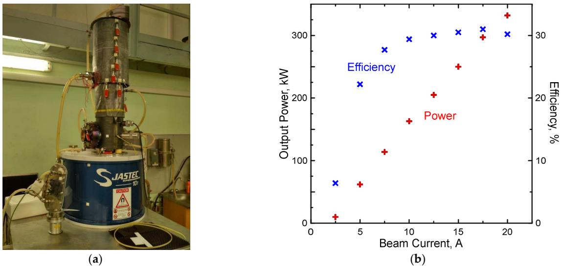
**Figure 1.** (a) General view of the 250 GHz gyrotron with TE<sub>19,8</sub> operating mode. (b) Experimentally obtained dependence of the output power and efficiency on the value of the beam current.
