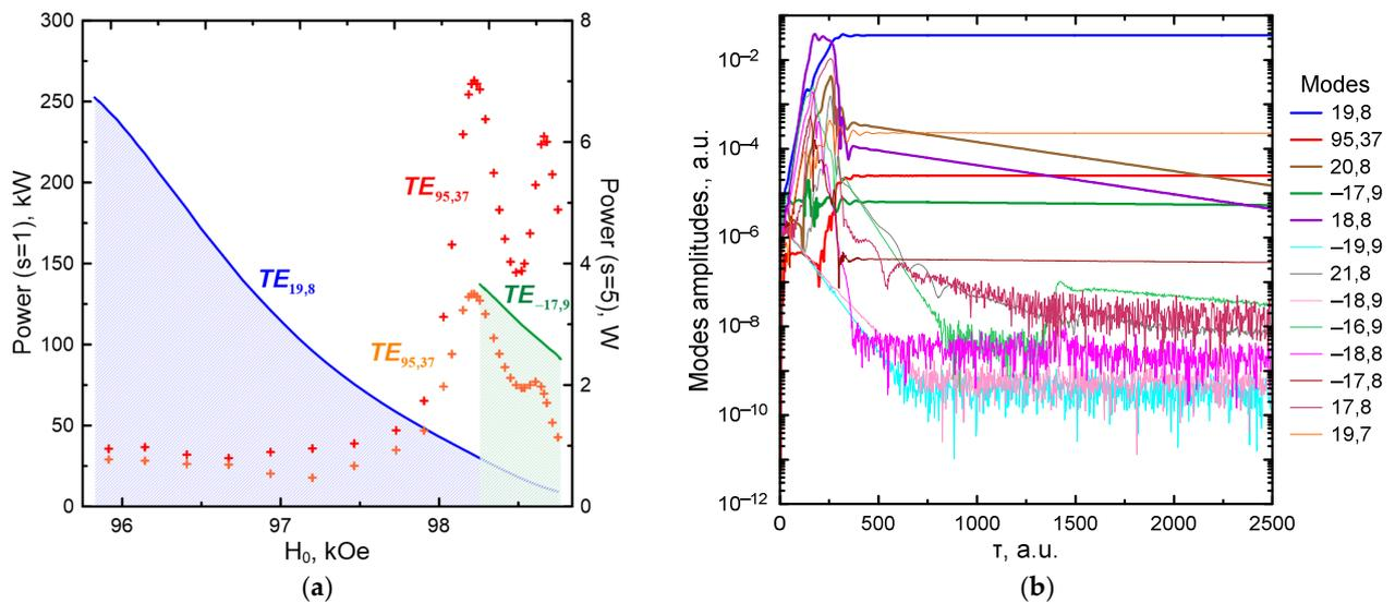
**Figure 2.** (a) Results of simulations for the 5th harmonic multiplication. Output power vs. guiding magnetic field for competing  $TE_{19,8}$  and  $TE_{-17,9}$  modes at the 1st cyclotron harmonic and for  $TE_{95,37}$  mode at the 5th cyclotron harmonic. Orange symbols depict the dependence of output power for the spread of electron velocities of 15%. (b) Establishment of the stationary oscillations in the process of competition between 12 modes at the fundamental cyclotron resonance.
