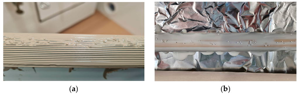
Figure 3. Introduction of the styrofoam balls (a) within the filler, adapted with permission from [19] and (b) on the filler layer within the coating.
