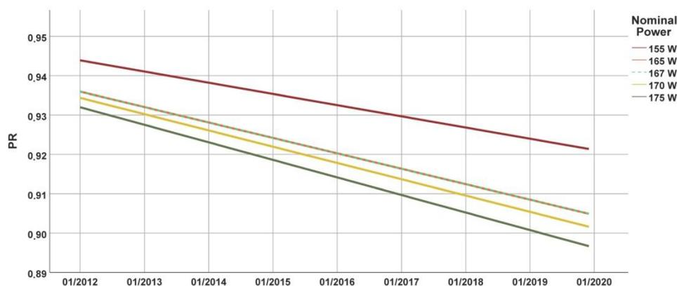
**Figure 6.** Variation of the PR for PV production units made with modules of 155 W to 175 W per elapsed month. Own elaboration.
