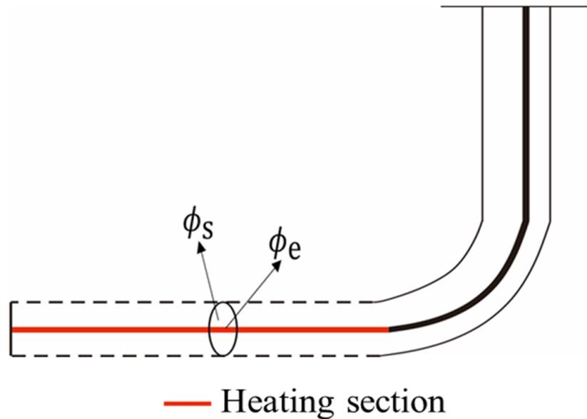
Figure 1. 2D cross-section map of horizontal wellbore during steam injection.
