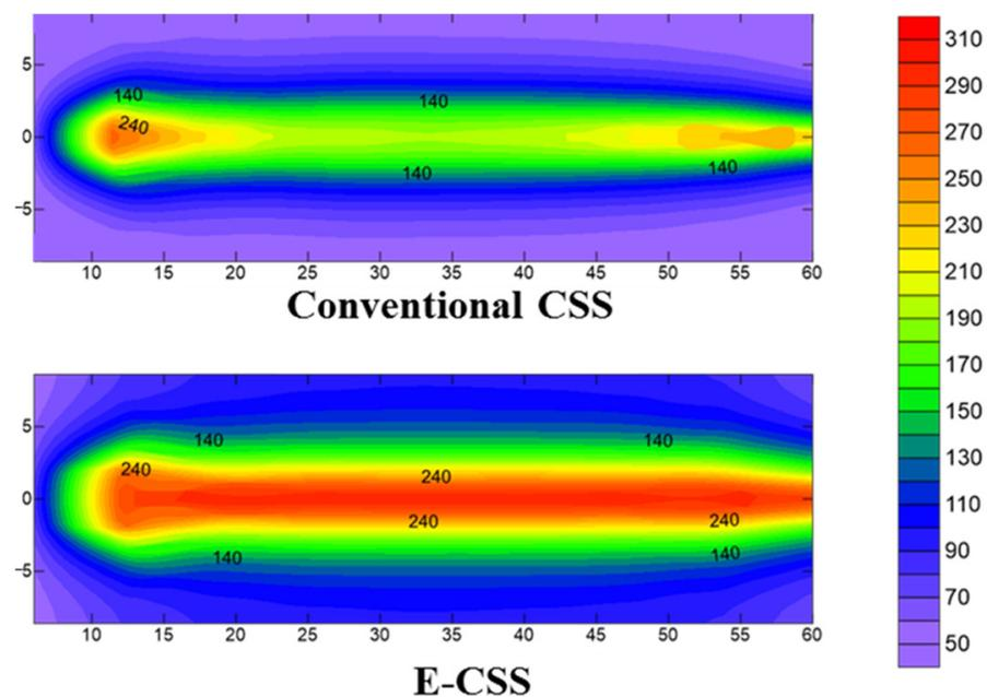
**Figure 4.** Temperature profile at the end of the second cycle steam injection.
