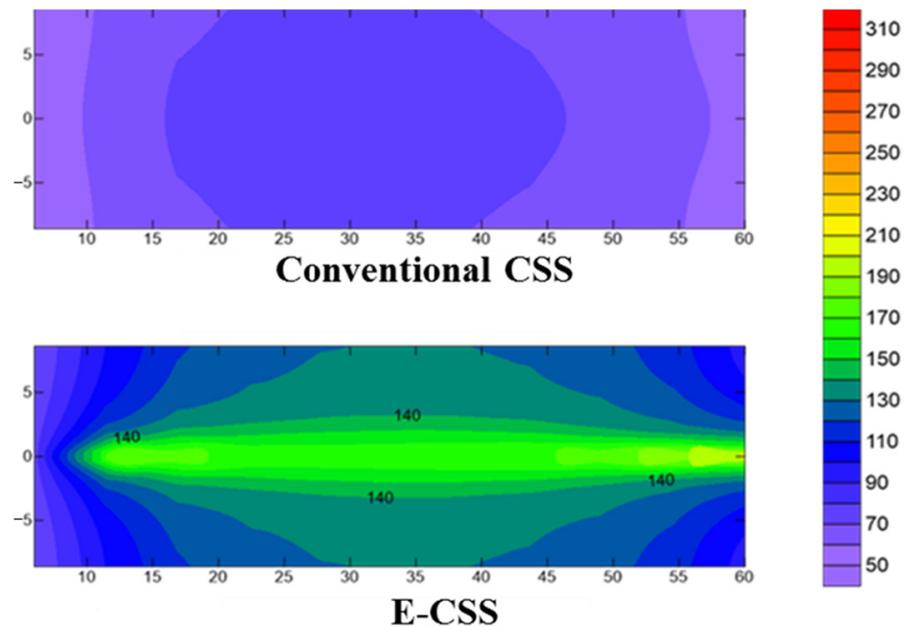
Figure 6. The comparison of the temperature field at the middle of the second cycle production phase.
