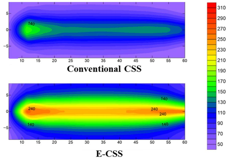
Figure 5. The comparison of the temperature field at the end of the second cycle soaking phase.
