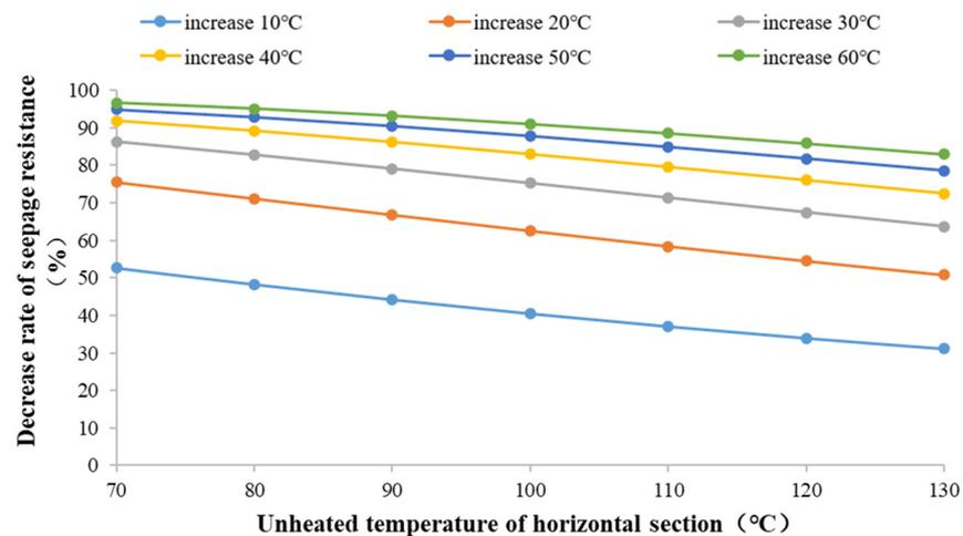
Figure 9. Wellbore porous flow resistance reduction ratio under different electrically enhanced temperatures.
