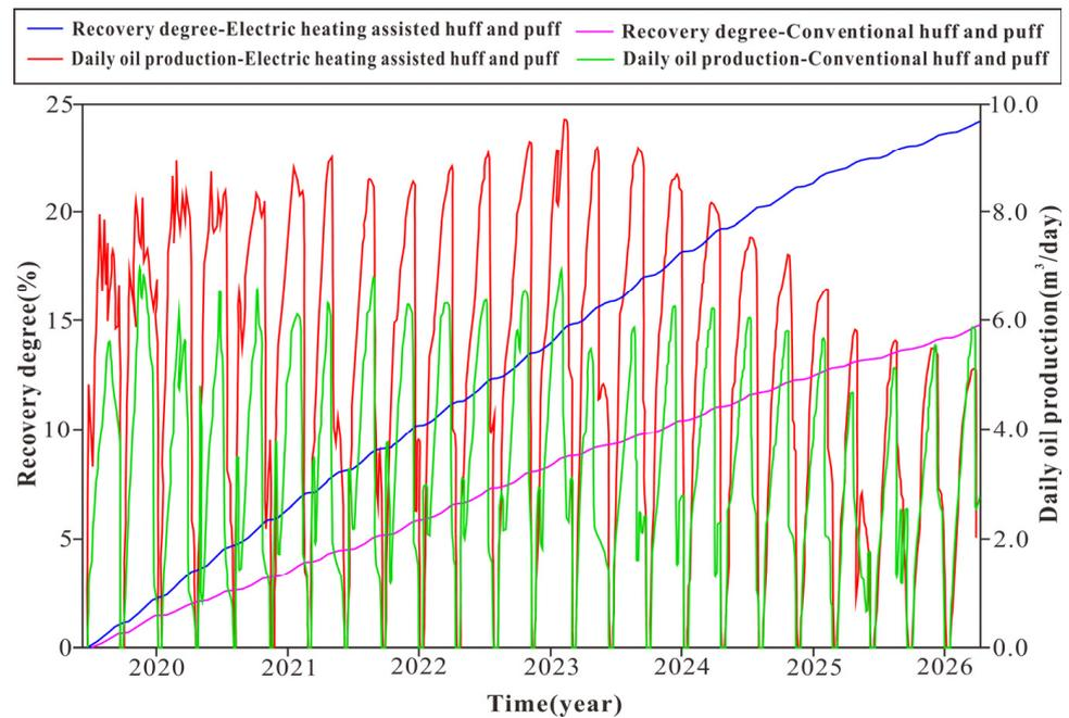
**Figure 10.** Comparison of oil rate and oil recovery factor for conventional CSS and E-CSS.
