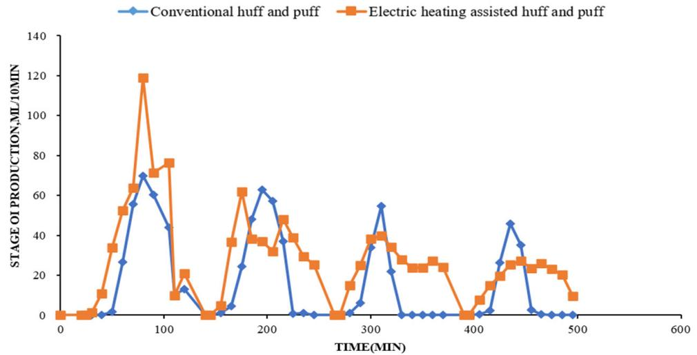
Figure 8. Comparison of oil production rate for conventional CSS and E-CSS.
