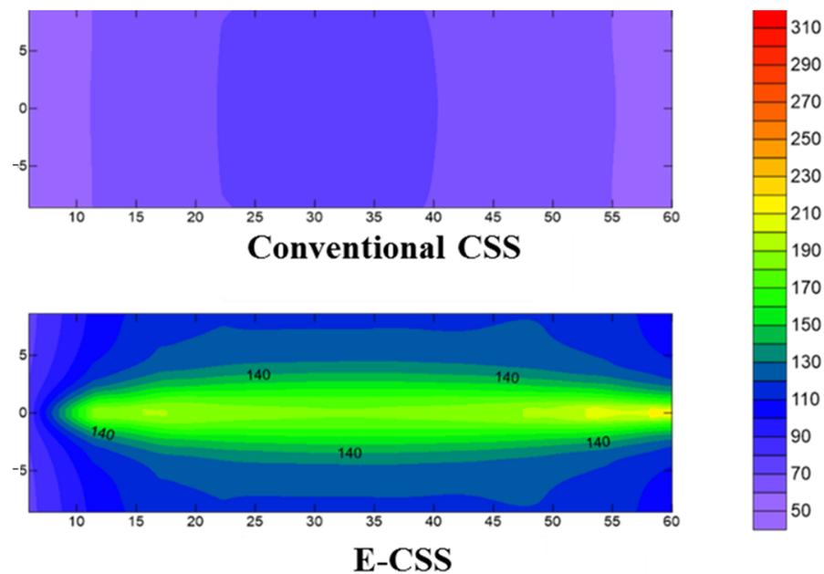
**Figure 7.** The comparison of the temperature field at the end of the second cycle production phase.
