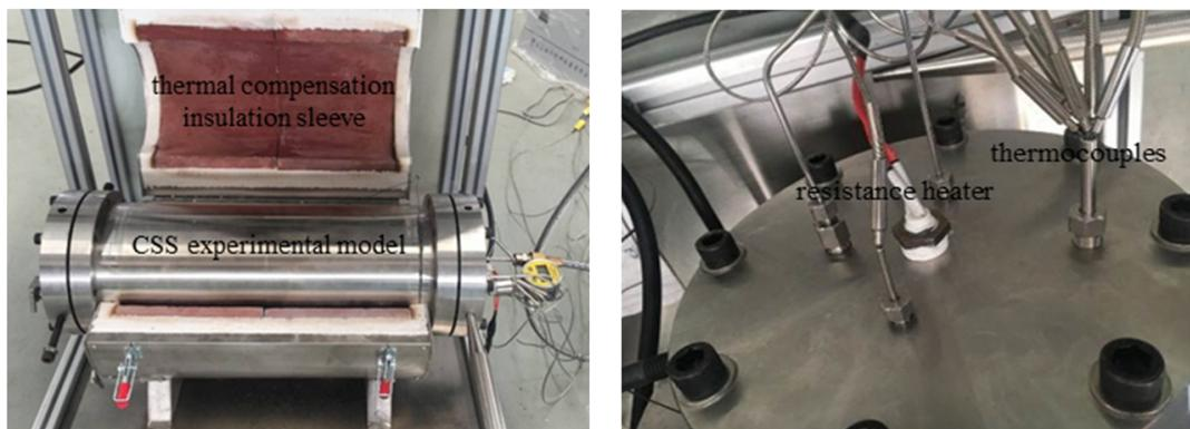
**Figure 2.** The experimental equipment of E-CSS: (a) schematic figure; (b) Physical picture.
