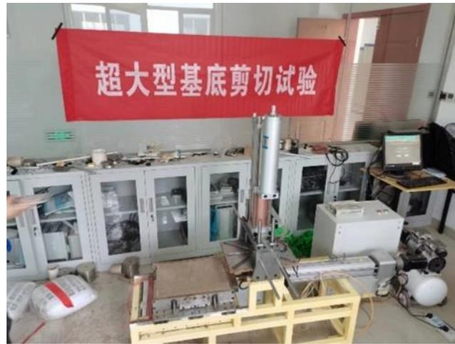
**Figure 6.** Ultra-large interface shearing equipment.
