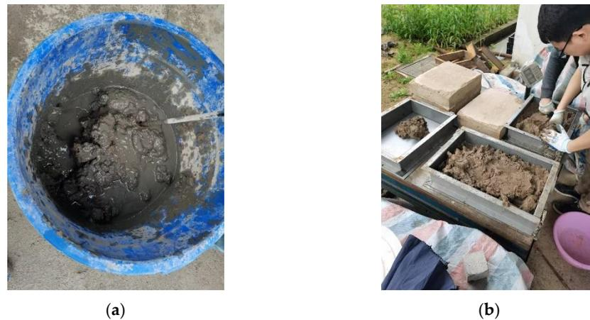
**Figure 2.** Preparation of the cement soil sample: (a) Cement soil mixing and (b) Cement soil formwork curing.
