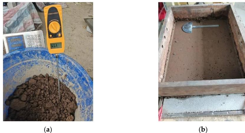
**Figure 5.** Preparation of the clay sample: (a) Moisture content measurement. and (b) Clay box.
