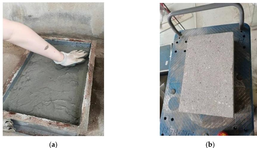
**Figure 1.** Preparation of the concrete test block: (a) Fabrication of the concrete test block and (b) Surface grinding of test block.
