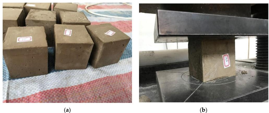
**Figure 3.** Strength characteristic test of the cement soil: (a) Preparation of the standard cubes. And (b) Unconfined compression test.
