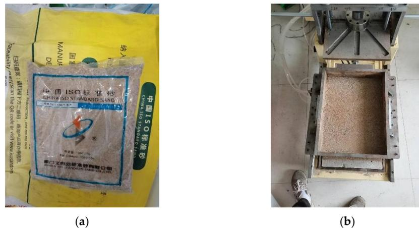
**Figure 4.** Preparation of the standard sand: (a) Standard sand unsealing and (b) Standard sand box.
