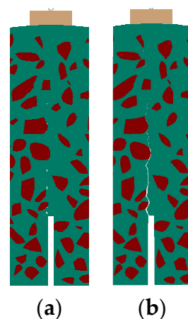
Figure 12. Crack propagation path at (a) -10\text{ }^{\circ}\text{C} ; (b) 0\text{ }^{\circ}\text{C} .
