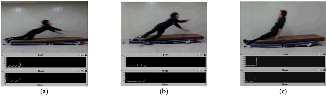
**Figure 2.** Photos performing 3 types of fall and their measured parameters, sum vector magnitude (SVM) and angle (Theta;  $\theta$ ). (a) Falling forward, (b) Falling sideways, (c) Falling backward.
