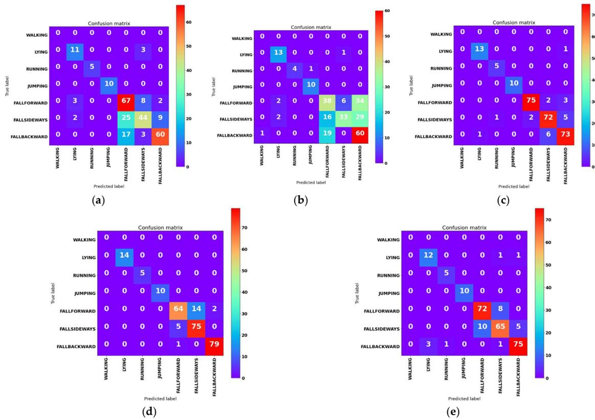
**Figure 6.** Confusion matrix applying 5-types of single parameter to the proposed LSTM-based fall detection system. (a)  $P_{\theta}$ , (b)  $P_S$ , (c)  $P_D$ , (d)  $P_G$ , (e)  $P_{GD}$ .
