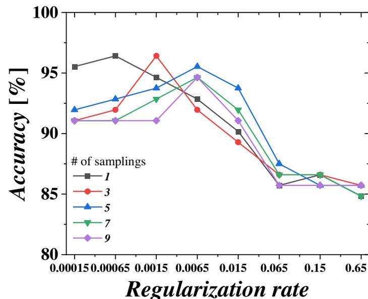
**Figure 11.** Validation data accuracy vs. regularization rate of the STM-LSTM-based fall detection system with respect to different sampling intervals.
