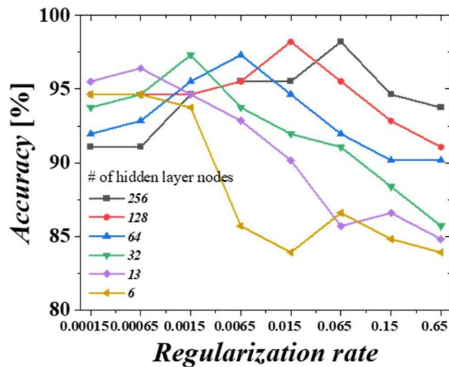
Figure 12. Validation data accuracy vs. regularization rate of the STM-LSTM-based fall detection system with respect to different number of hidden layer nodes.
