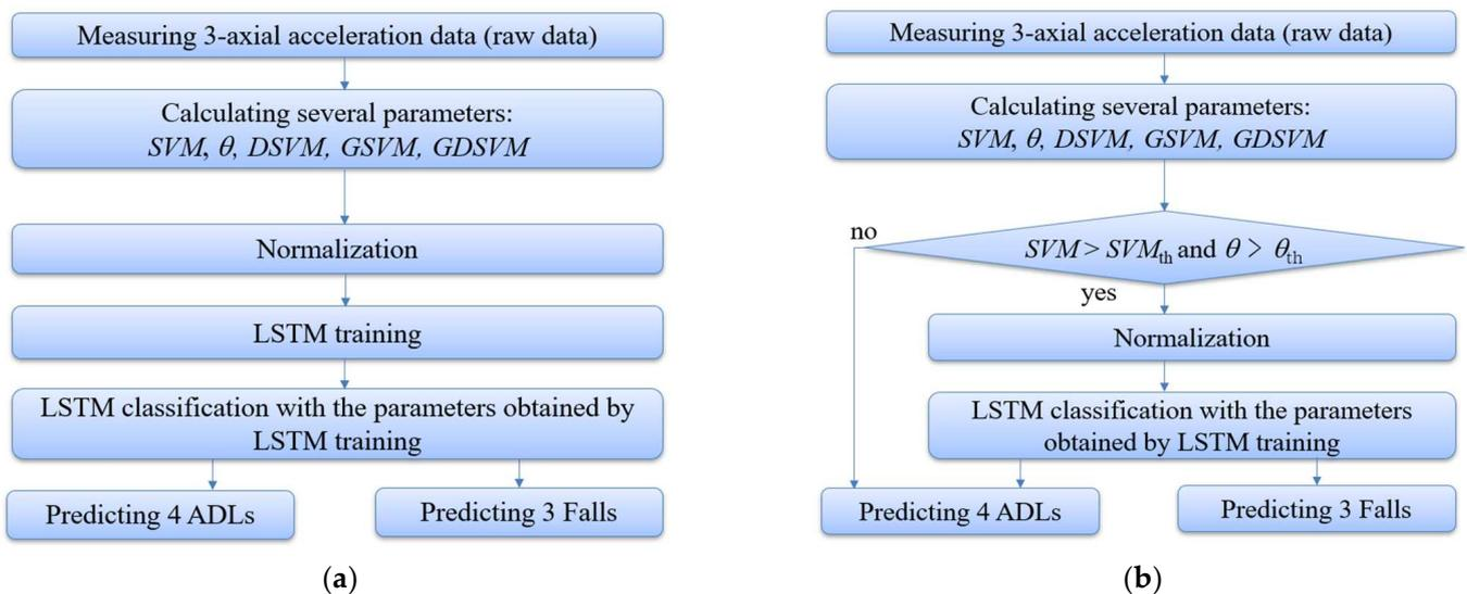
**Figure 3.** Flow charts of the proposed fall detection system. (a) Training mode and (b) test mode.
