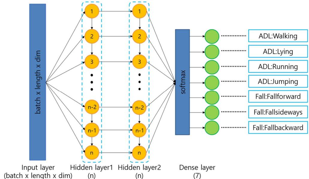
**Figure 5.** Fall detection model architecture for LSTM.
