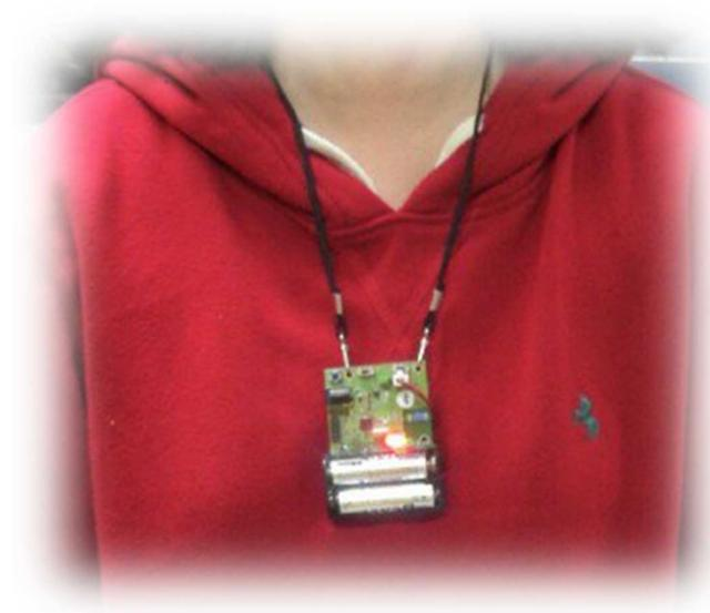
**Figure 1.** Photo of a person wearing a real edge device as a pendant to participant's neck for implementing the proposed fall detection system.
