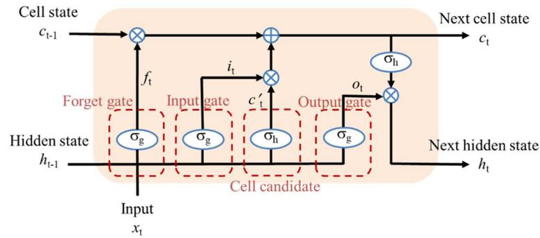
**Figure 4.** The typical structure of long-short term memory (LSTM).  $\sigma_h$  and  $\sigma_g$  denote the hyperbolic tangent and sigmoid functions, respectively.
