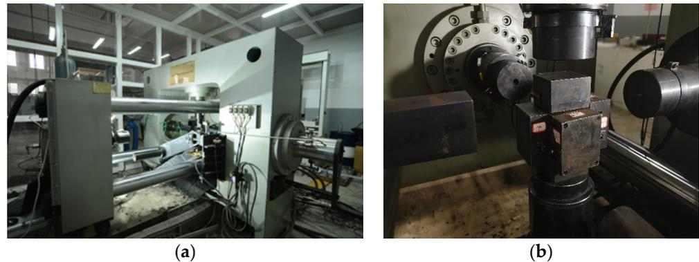
**Figure 1.** True triaxial coal-rock dynamic behavior testing system: (a) schematic diagram of equipment; (b) single face unloading part with a droppable loading bar.
