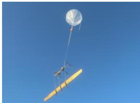
Figure 18. The rise of balloon-borne solar-powered UAV.
