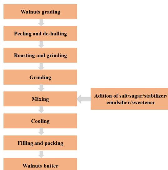
**Figure 1.** Flow diagram of walnuts butter production.
