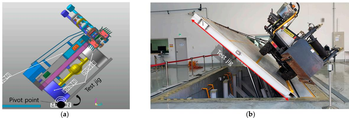
**Figure 5.** The conditions of the rollover test for tilt angle: (a) simulation of the lateral overturning and (b) validation test of the lateral overturning of the radish harvester.
