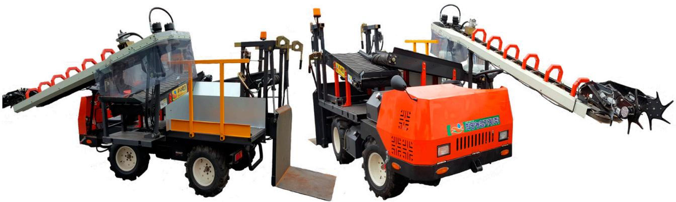
**Figure 1.** The self-propelled radish harvester used in this study.
