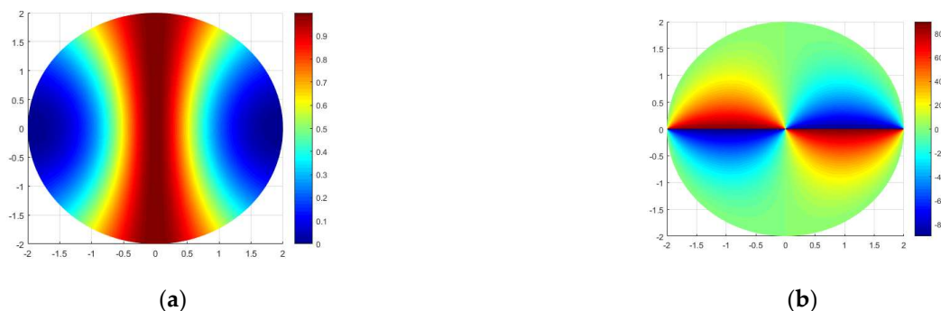
Figure 7. 2-D polarization distribution characteristics of sky complex spherical projection, (a) Polarization degree (b) Polarization angle.
