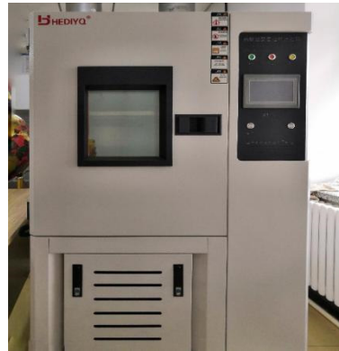
Figure 2. The thermostatic chamber of constant humidity. (Shanghai Hengding Instrument & Equipment Factory, HDGDSJ-150).
