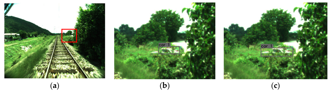
Figure 6. Example of improved object bounding box coordinates. (a) Original image with marked region containing the considered object (red rectangular). (b) Magnified predictions of Model 1. (c) Magnified predictions of Model 2.
