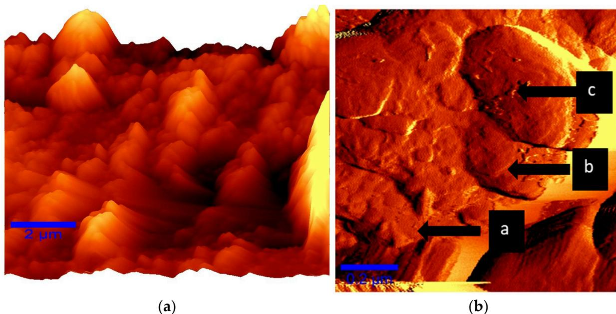
**Figure 5.** AFM-Raman deposition profile studies: (a) Random PV glass sector analysis; (b) soiling layers growing one over the other on the lower part of the PV glass.
