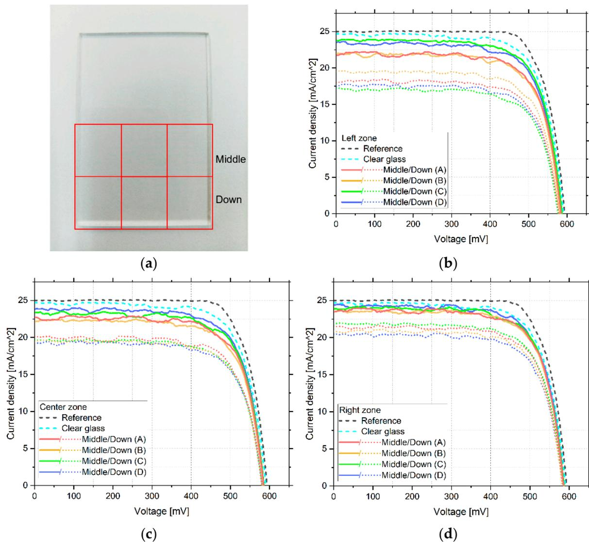
**Figure 6.** IV curve measurement of the lower and middle parts of glass samples (A, B, C, and D). (a) Clean glass divided into sectors to be analyzed; (b) IV curves on the middle and lower left sides; (c) IV curves on the middle and lower central parts; and (d) IV curves on the middle and lower right side.
