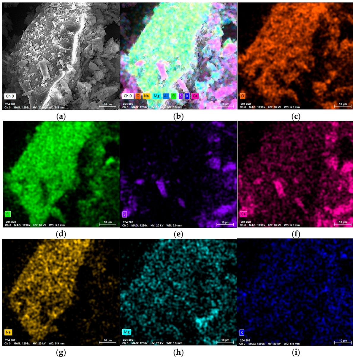
**Figure 4.** Elemental mapping analysis on a random section of the soiling samples deposited on the exposed glass. (a) Randomly selected area to be analyzed. (b) Combination of elements present in selected area (O, Na, Mg, Al, Si, S, K and Ca). (c–i) Mapping of the elemental analysis to random section of soiling samples deposited on the exposed glass.
