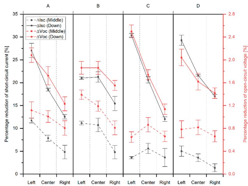
**Figure 7.** Short-circuit current and open-circuit voltage percentage reduction for the samples (A–D).
