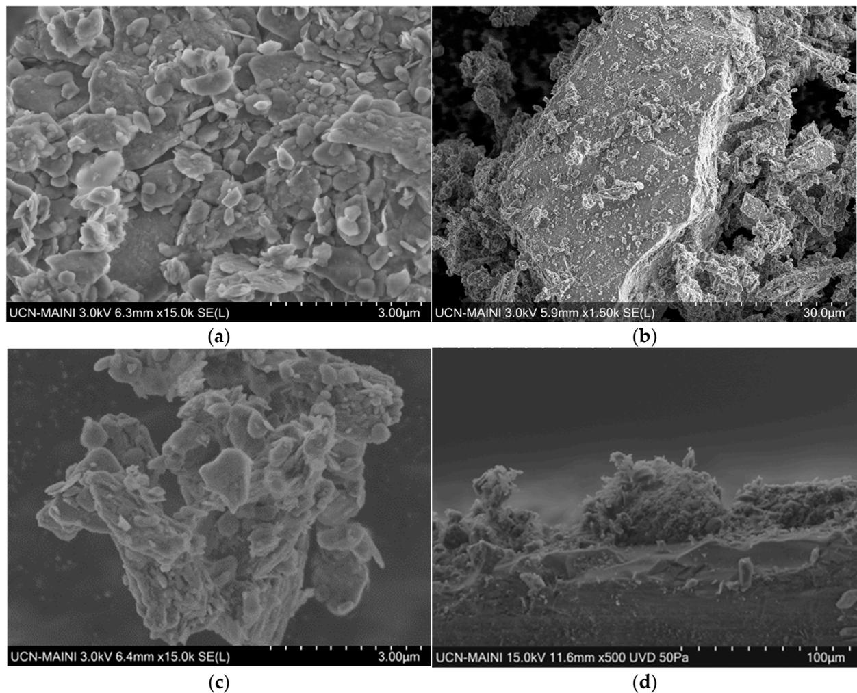
**Figure 3.** Scanning electron microscopy: (a) Sample of soiling deposited on the lower part of the PV glass; (b,c) random prismatic particle analysis; and (d) PV glass cross-section.
