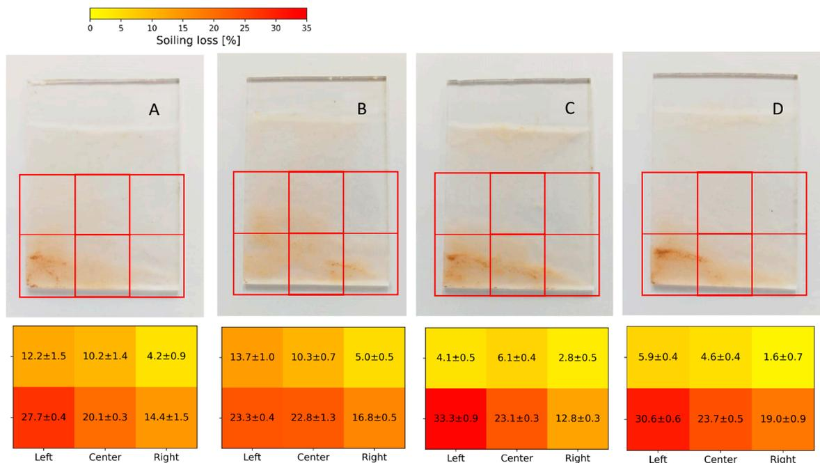
**Figure 8.** Power reduction percentage of glass samples (A–D) installed northwards at PSDA at a 20° slope for a one-year exposure (September 2020–2021).
