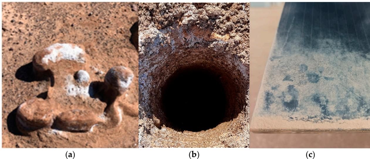
**Figure 2.** Site geology influence on PV module material deposition: (a) Random picture of PSDA soil; (b) Pit 5; and (c) material deposited on the fine layer module at PSDA.
