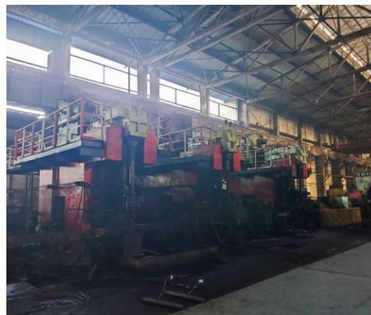
**Figure 2.** Photograph of the rough rolling mill.
