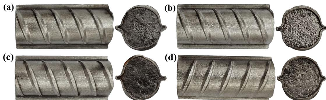
**Figure 14.** Surface morphologies of various rebars after rust removal: (a) 20MnSiV/316L rebar; (b) 35#/316L rebar; (c) 45#/316L rebar; (d) 55#/316L rebar.
