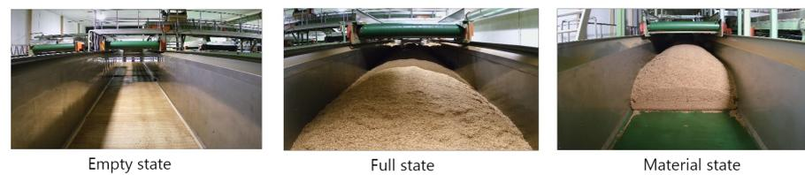
Figure 3. Tobacco cabinet data. The left is the empty state, the middle is the full state, and the right is the material state.
