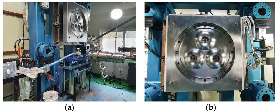
**Figure 10.** The overall APG system (a); and the mold for GIS spacer (b).
