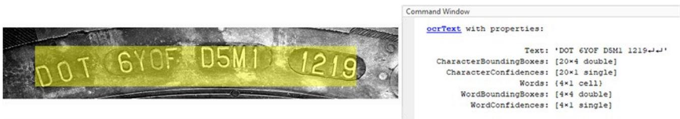
**Figure 9.** Result of verification process via optical character recognition (OCR) function.
