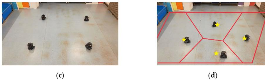
**Figure 18.** Diamond formation experiment: (a) density function distribution; (b) cost function; (c) initial position; (d) final position.
