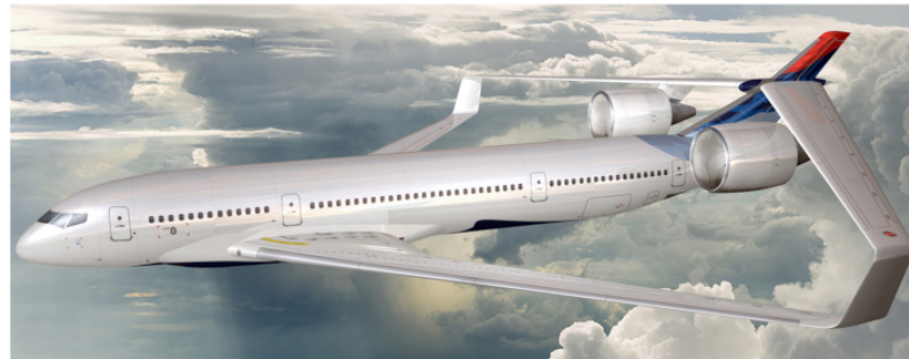
Figure 1. Box-Wing Aircraft (BWA) design from Lockheed Martin (with NASA courtesy).
