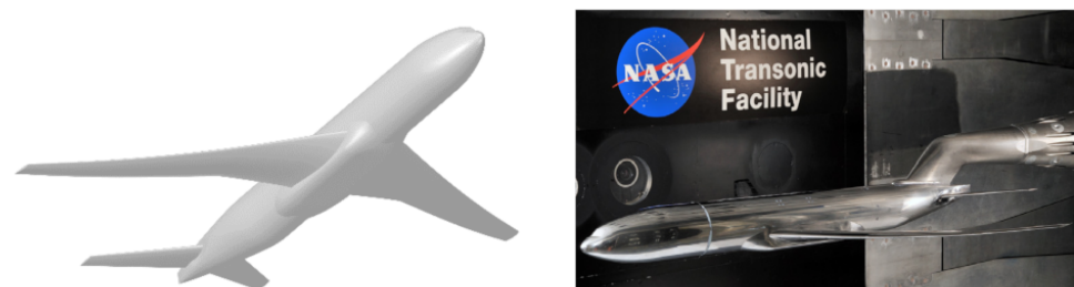
Figure 3. Common Research Model (CRM) aircraft in its original wing-body-tail (WBT) configuration (i.e., with horizontal tail only). CAD model (left) and small-scale experiment ((right), reproduced from [47] with NASA courtesy).
