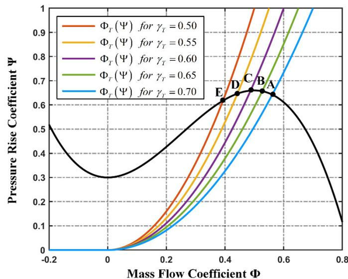
Figure 3. The characteristic curves of compressor and throttle.
