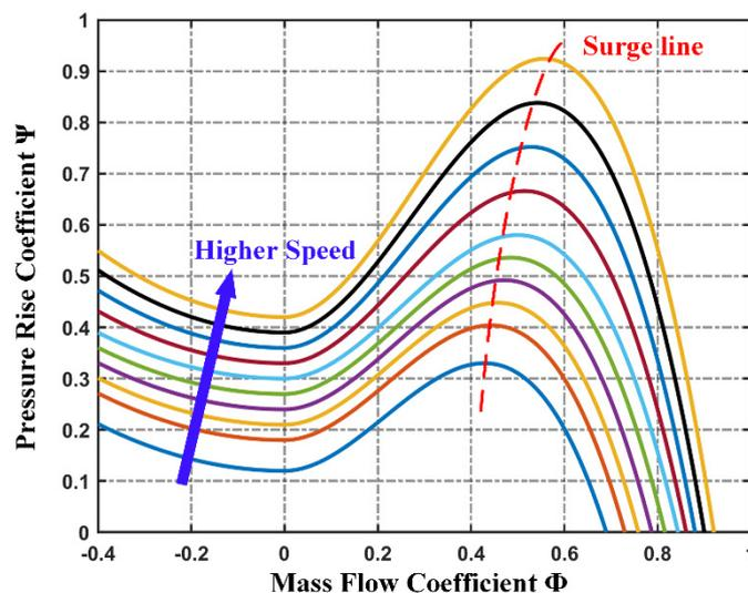
Figure 7. Compressor characteristic curves cluster.
