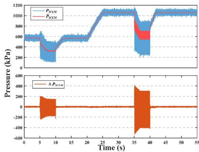
**Figure 15.** The steady-state pressure component  $\bar{P}_{3CLM}$  and the pulsating pressure component  $\Delta P_{3CLM}$  of simulated pressure  $P_{3CLM}$ .
