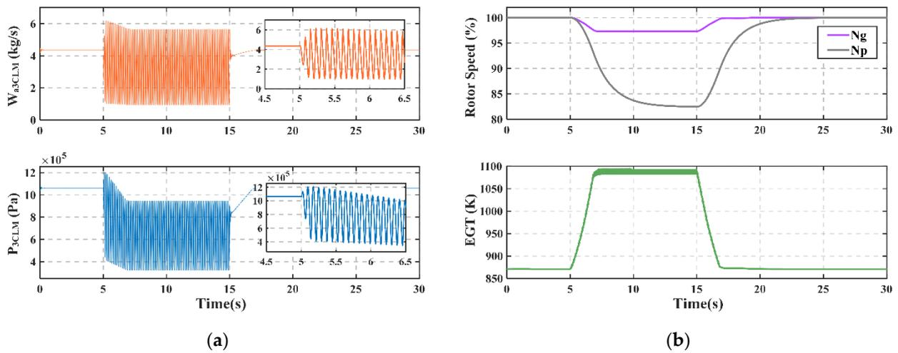
Figure 10. Simulation of surge dynamic process at design point: (a) The mass flow and pressure at compressor outlet; (b) Engine's rotor speed and exhaust temperature.
