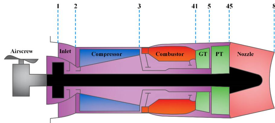
Figure 1. The layout of turboshaft engine.
