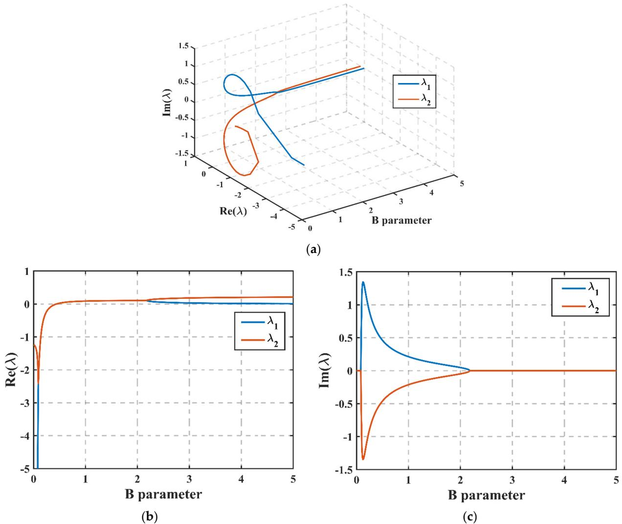
**Figure 4.** The Variation of eigenvalue trajectories with  $B$  parameter: (a) Variation of two eigenvalues; (b) Variation of real part of two eigenvalues; (c) Variation of imaginary part of two eigenvalues.
