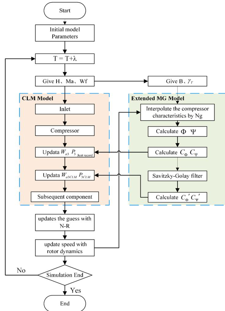
Figure 9. Dynamic calculation of real-time surge model of turboshaft engine.
