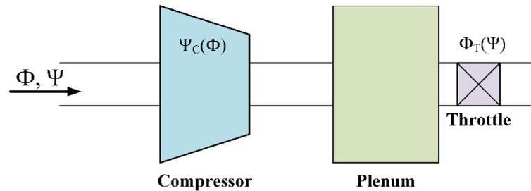
Figure 2. Schematic diagram of the compression system.
