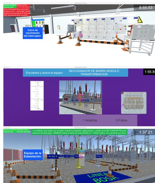
**Figure 7.** Three different missions can be performed. The top image shows indoor medium-voltage switchgear maintenance on an outgoing feeder including CB switching operation and CB withdrawal and reconnection after maintenance. The middle image shows outdoor yard equipment recognition according to one-line diagram. The bottom image shows an HV switchgear bay local operation of non-load disconnector.
