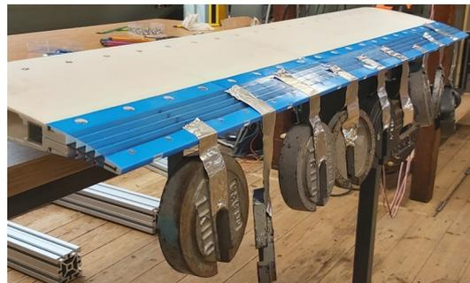
**Figure 18.** FishBAC device loaded with point masses (proof load). The wing was clamped by the spar using two vices.
