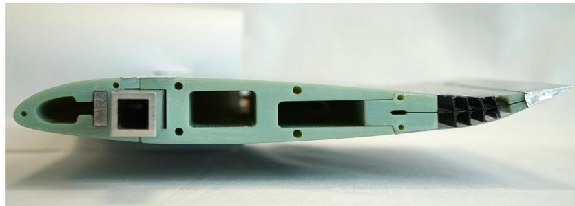
**Figure 2.** Second generation of FishBAC devices designed around a carbon fibre composite spine [23]. The copyright of this photograph belongs to Andres E. Rivero (co-author of this article), and has been used with his permission.
