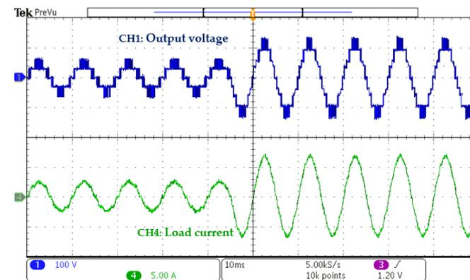
**Figure 18.** Output voltage (CH1) waveform at an increasing load current (CH4).
