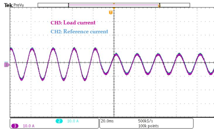
Figure 19. Load current (CH3) waveform at a decreasing reference current (CH2).
