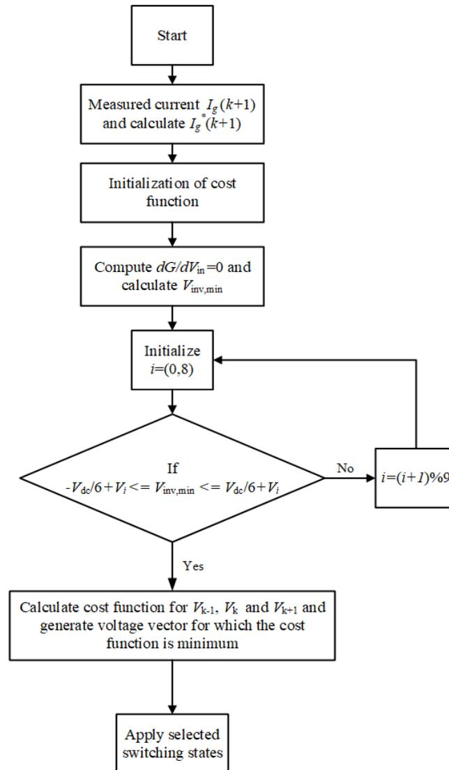
Figure 3. Flowchart of modified MPC optimized algorithm.
