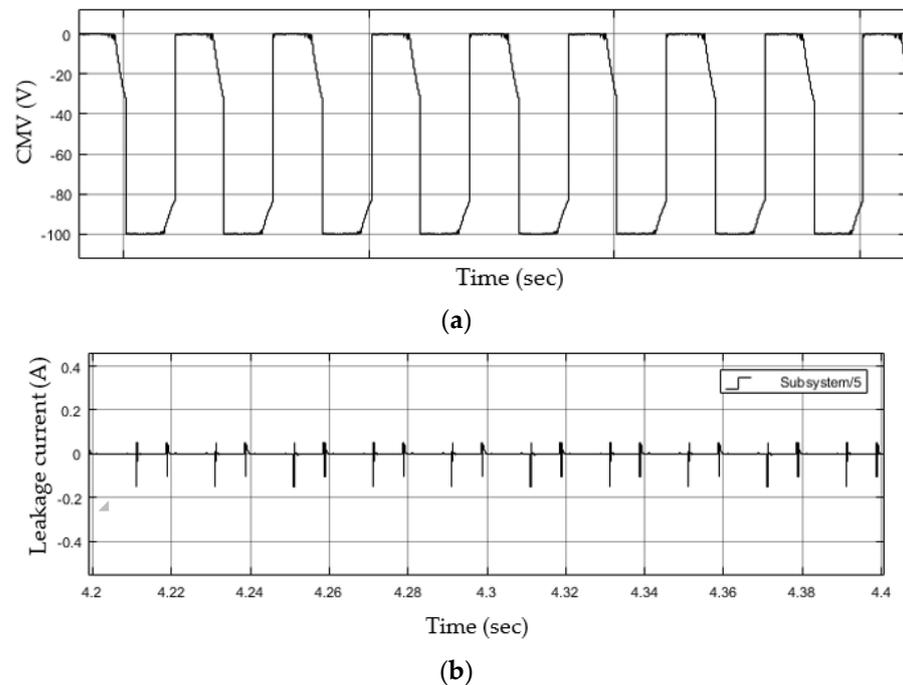
**Figure 11.** Simulation results HMLI: (a) common mode voltage in grid connected HMLI, and (b) leakage current.
