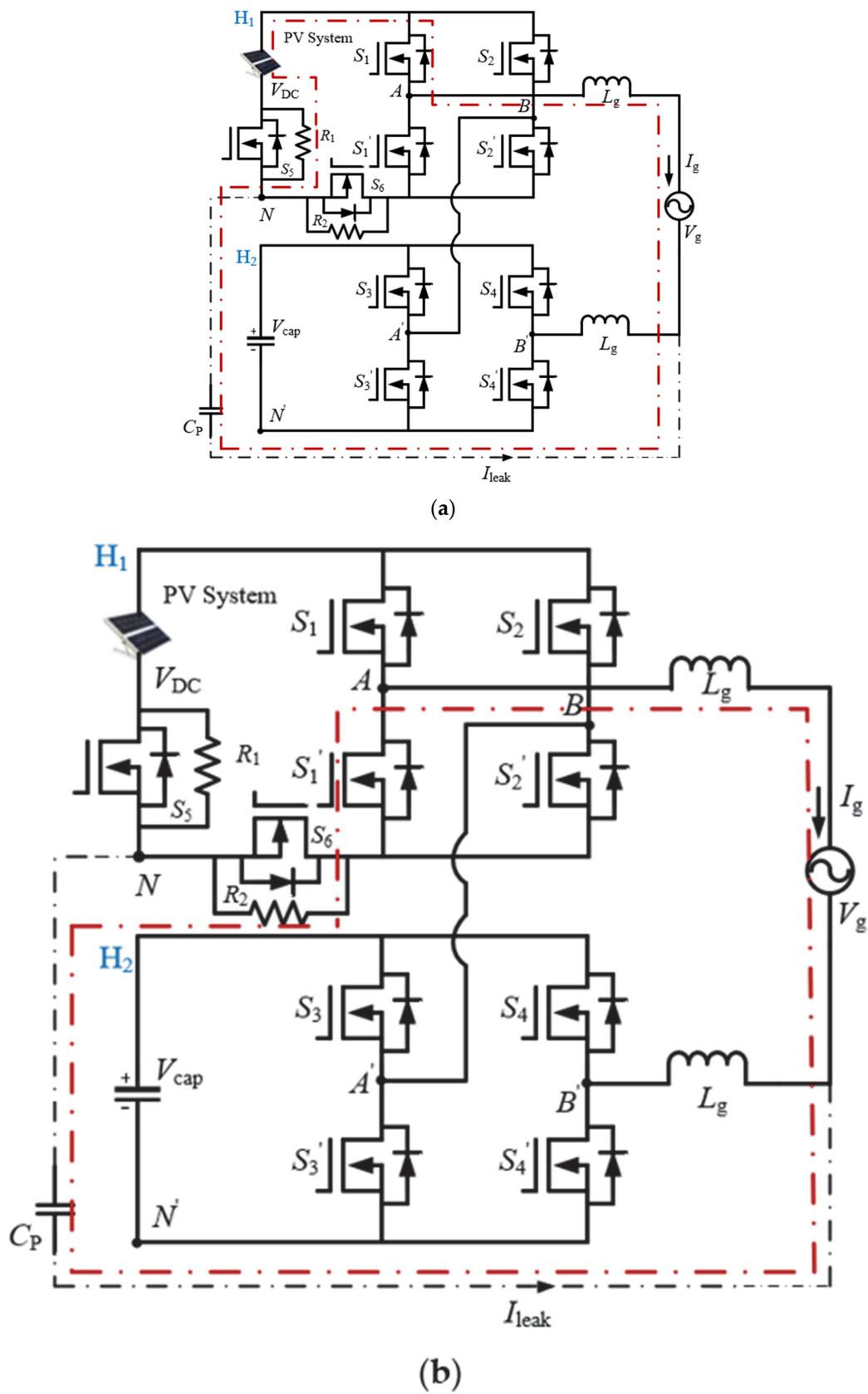
Figure 5. Leakage current path: (a) through  $S_5$  ( $R_1$ ), and (b) through  $S_6$  ( $R_2$ ).
