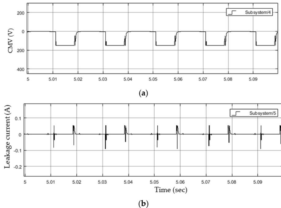
Figure 8. Simulation results of HMLI (enabled TC): (a) common mode voltage, and (b) leakage current.
