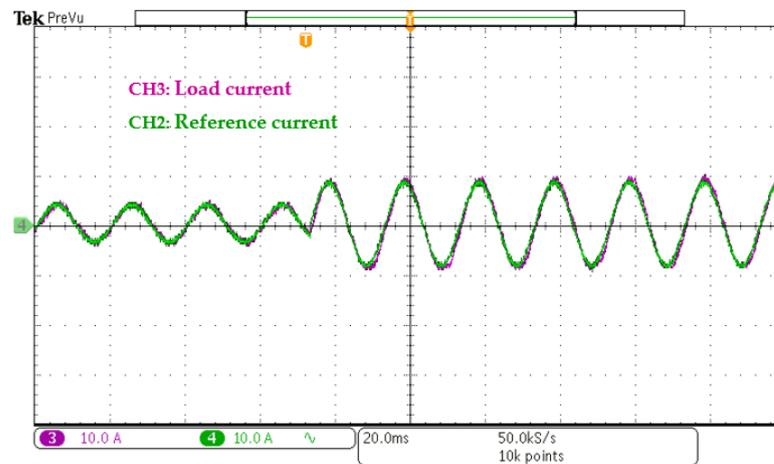
Figure 20. Load current (CH3) waveform at an increasing reference current (CH2).
