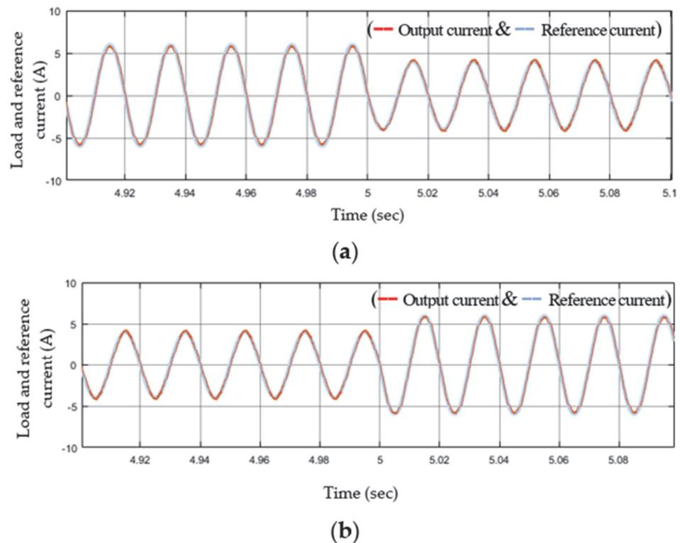
**Figure 9.** Dynamic results of HMLI: (a) load current tracking when decreasing the reference current, and (b) load current tracking when increasing reference current.
