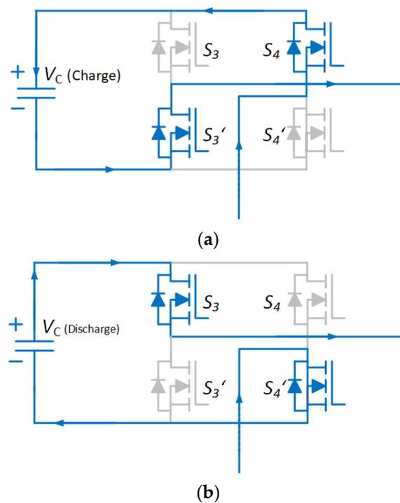
**Figure 4.** Capacitor voltage balancing: (a) charging intervals, and (b) discharging intervals.
