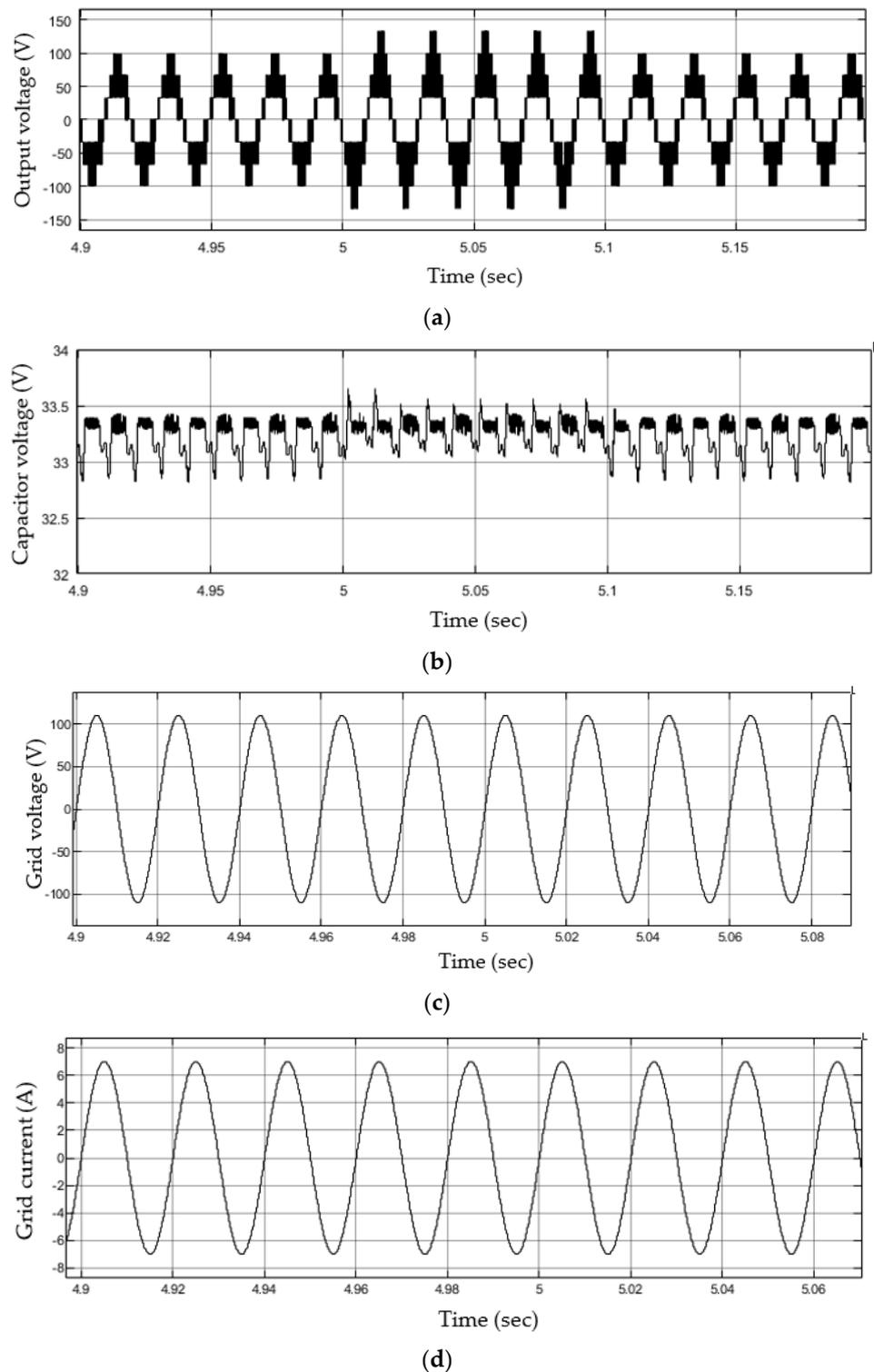
**Figure 10.** Simulation results of HMLI: (a) grid voltage dynamics of HMLI, (b) capacitor voltage balancing, (c) Grid voltage, and (d) grid current.
