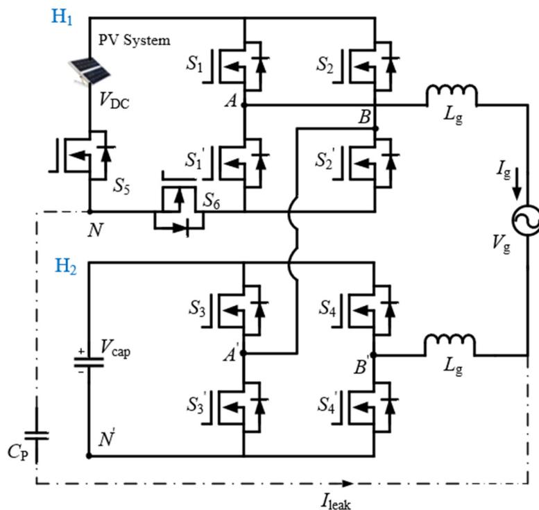
Figure 1. Transformer less nine-level PV-supported HMLI.
