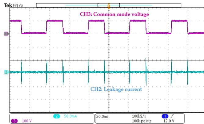
Figure 14. Common mode voltage (CH3) and leakage current (CH2) waveform.
