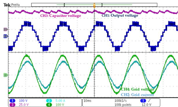
**Figure 16.** HMLI output voltage (CH1), capacitor voltage (CH3) and grid voltage (CH4), and grid current (CH2) waveforms.
