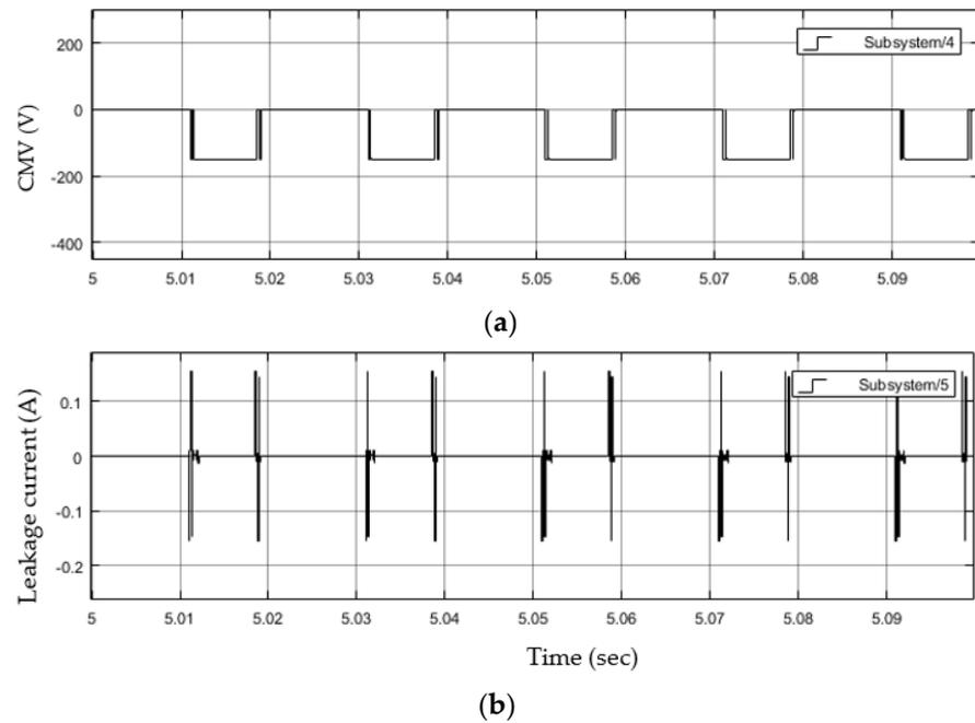
Figure 7. Simulation results of HMLI (disabled TC): (a) common mode voltage, and (b) leakage current.
