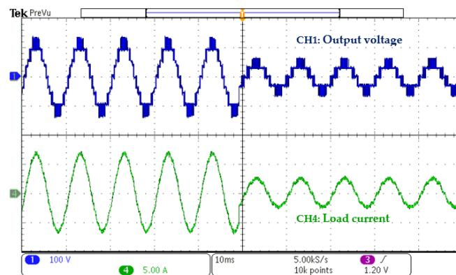
**Figure 17.** Output voltage (CH1) waveform at a decreasing load current (CH4).
