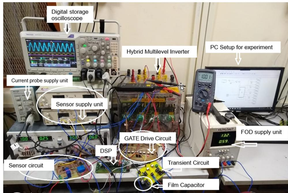
Figure 12. Photograph of the experimental setup.
