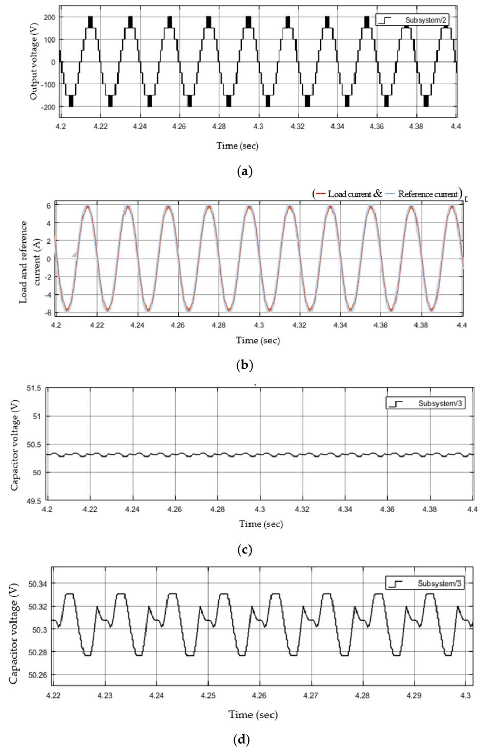
**Figure 6.** Simulation results of HMLI: (a) output voltage waveform, (b) load current tracking (— output current & — reference current), (c) capacitor voltage with voltage balancing, and (d) capacitor voltage charging and discharging.
