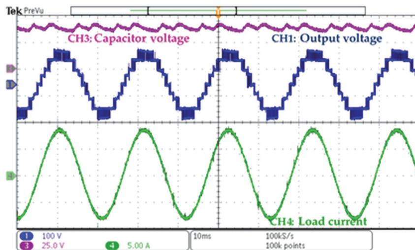
Figure 13. HMLI output voltage (CH1), capacitor voltage (CH3), and load current (CH4) waveform.
