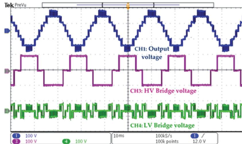
Figure 15. HMLI output voltage (CH1), high-voltage bridge voltage (CH3), and low-voltage bridge voltage (CH4) waveforms.
