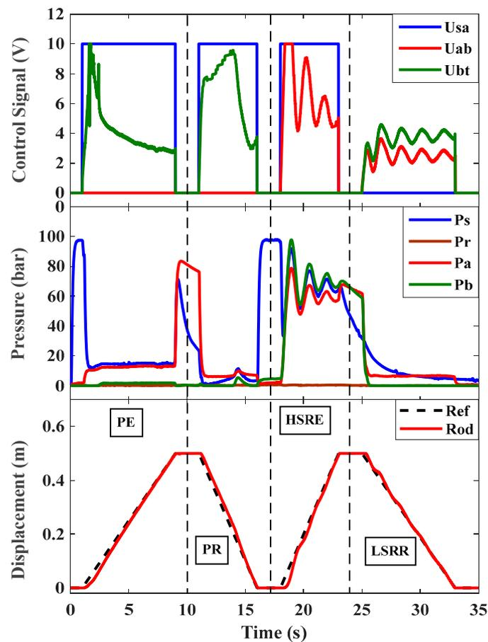
**Figure 6.** The NIMV experimental results.  $U_K$  ( $K = sa, ab$  or  $bt$ ): control signal of  $K_{sa}$ ,  $K_{ab}$ , and  $K_{bt}$  valves.  $P_s$ : pressure at pump outlet;  $P_a$ ,  $P_b$ : pressure at bore and rod chamber of cylinder,  $P_r$ : pressure at tank.
