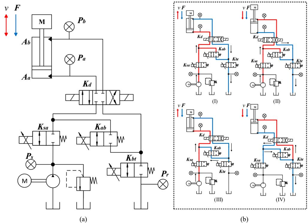
**Figure 2.** (a) Configuration of an actuator using the new IMV circuit. (b) Four metering modes of the NIMV; (I) PE mode; (II) PR mode; (III) HSRE mode; (IV) LSRR mode.
