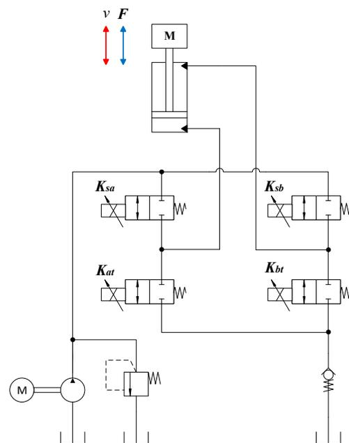
**Figure 1.** The conventional independent metering valve system.
