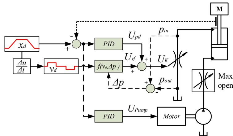
Figure 4. Working principle of valve and pump control.
