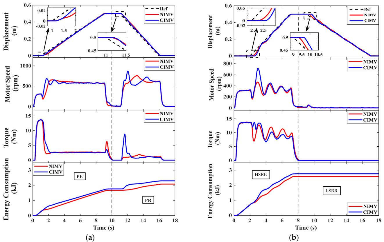
**Figure 7.** Comparison of the operation between the NIMV and CIMV systems in both cycles. (a) Cycle 1; (b) Cycle 2.
