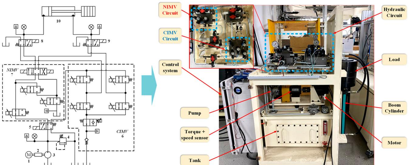
Figure 5. The test bench of the hydraulic excavator boom system.
