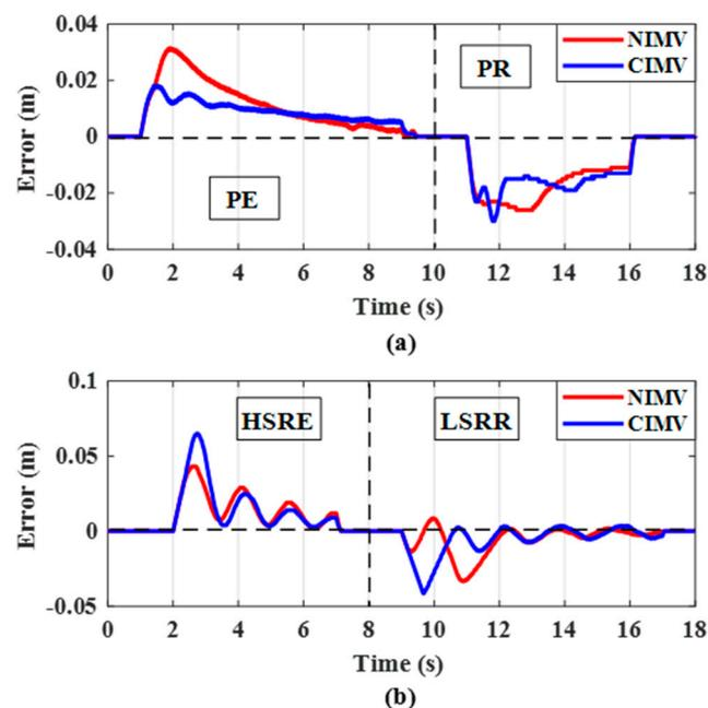
**Figure 8.** Comparison of the displacement errors in the NIMV and CIMV systems. (a) Cycle 1; (b) Cycle 2.
