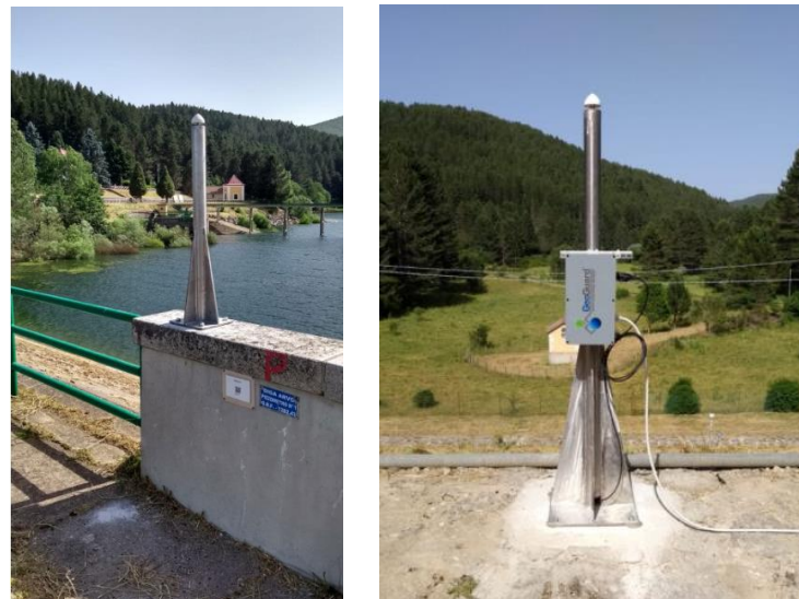
Figure 2. Steel pillars supporting the antennas for points PT3 (left) and PT4 (right). The other points are materialized with the same kinds of structures.
