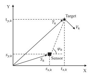
Figure 1. Schematic diagram of 2D bearing-only TMA.
