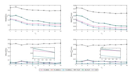
**Figure 12.** Time-averaged RMSEs, BNorms and bearing noise standard deviation at V = 0.2 m/s for the PL-MMSE, PLKF, BC-PLKF and IVKF algorithms, as well as, the PL-MMSE algorithm with nonlinear constraints proposed in the paper.
