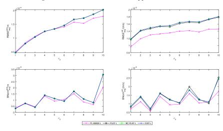
**Figure 11.** Time-averaged RMSEs, BNorms and bearing noise standard deviation at  $V = 10^{-4}$  m/s for the four algorithms combined with the second-order approximation method.
