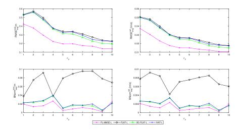
**Figure 15.** Time-averaged RMSEs, BNorms and bearing noise standard deviation at V = 0.2 m/s for the four algorithms combined with the second-order approximation method.
