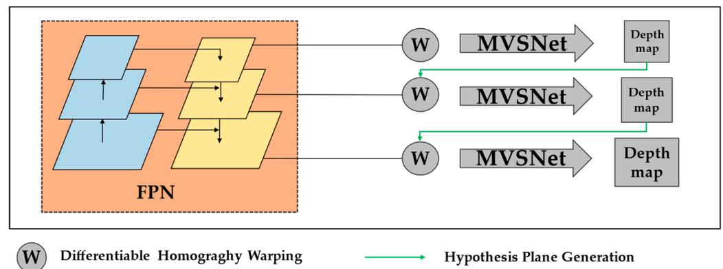
Figure 4. Coarse-to-fine computational deep MVS network.
