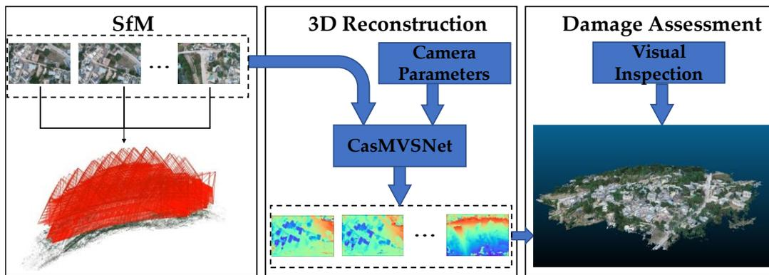
Figure 2. Workflow of building damage classification based on 3D model.
