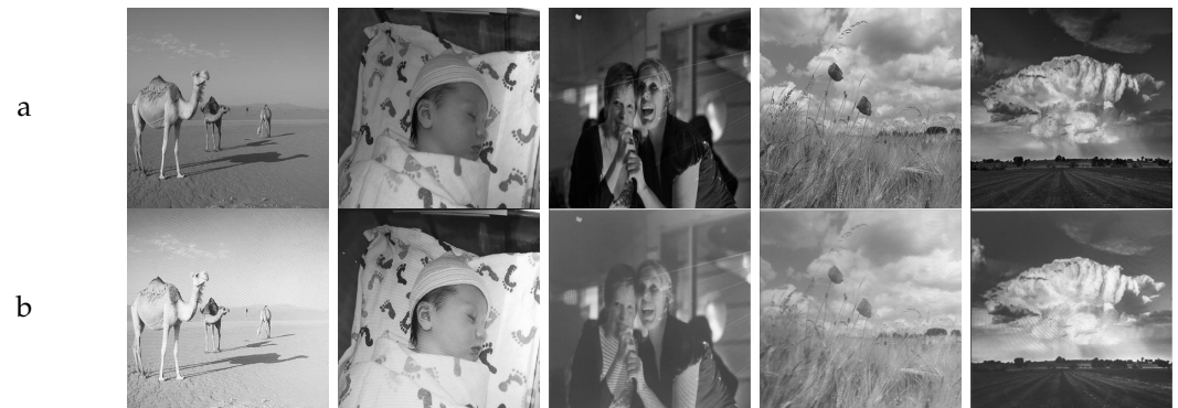
Figure 8. Moiré pattern test results from COCO 2014 gray dataset by the fine-tune network. (a) pure images; (b) images (512 × 512) with moiré pattern.
