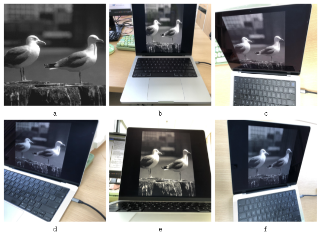
Figure 1. Real leak cases: (a) original image, (b) screen-shooting image with front view, (c) screen-shooting image with vertical perspective angle (up), (d) screen-shooting image with horizontal perspective angle (right), (e) screen-shooting image with vertical perspective angle (down), (f) screen-shooting image with horizontal perspective angle (left).
