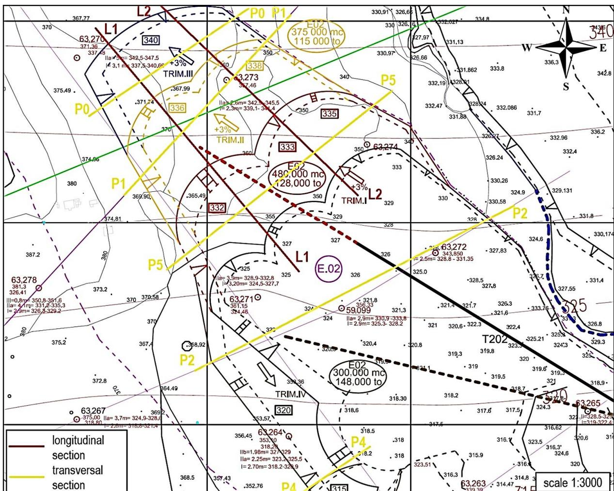
Figure 6. Evolution of Oletu open pit and the longitudinal and cross sections [56].
