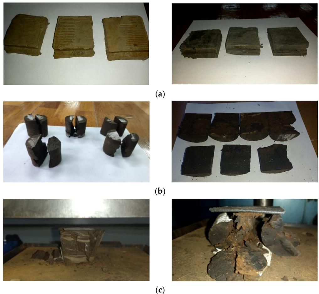
**Figure 5.** Laboratory tests: (a) direct shearing tests on yellow-brown clay and sandy marl; (b) shearing tests on lignite (mandatory planes); (c) uniaxial compression and traction (Brazilian method) on lignite [65].
