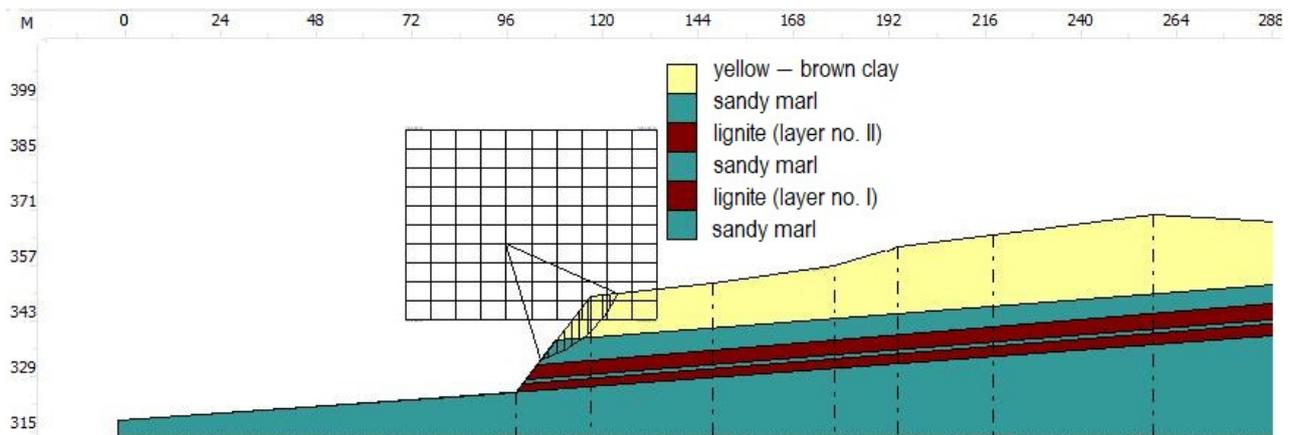
**Figure 11.** Section L1–Stability analysis for the proposed design.
