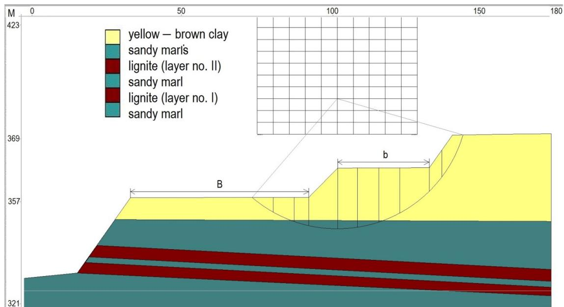
**Figure 13.** Section P1—Stability analysis of the sub-steps system (excavated in yellow-brown clay).
