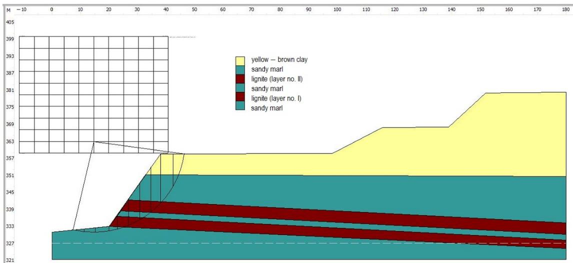
**Figure 12.** Section P1—Stability analysis of the lower excavation step.
