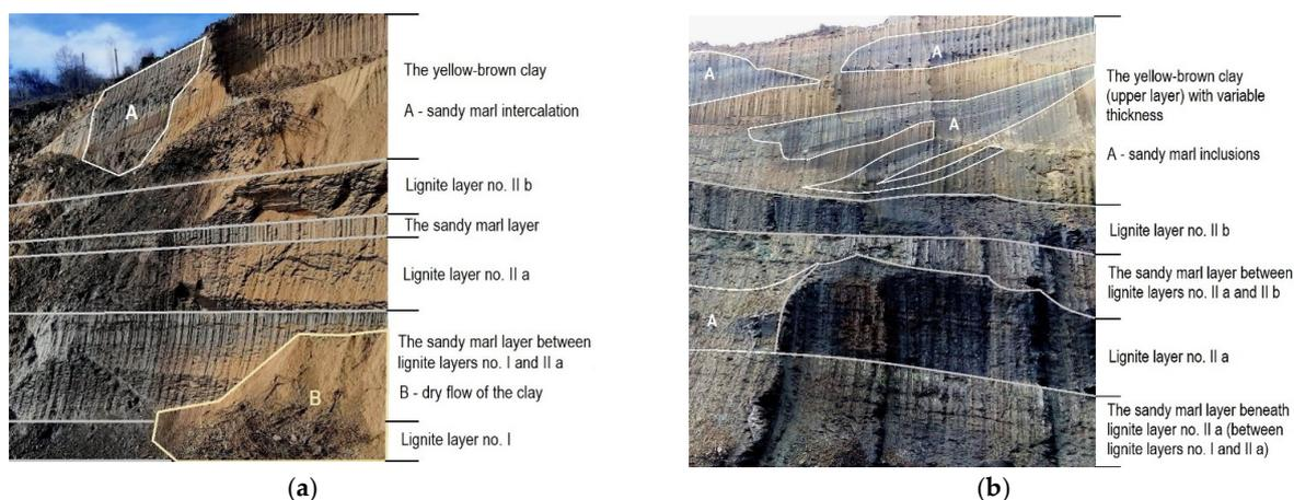
**Figure 4.** (a) The alternation of rock layers; (b) the discontinuity of rocks with variable thicknesses (the pictures were taken at different moments in time, in different weather conditions and from different distances and angles relative to the working front).
