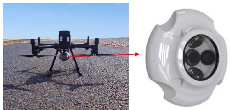
Figure 5. UAV for sand accumulation air survey and camera lens.
