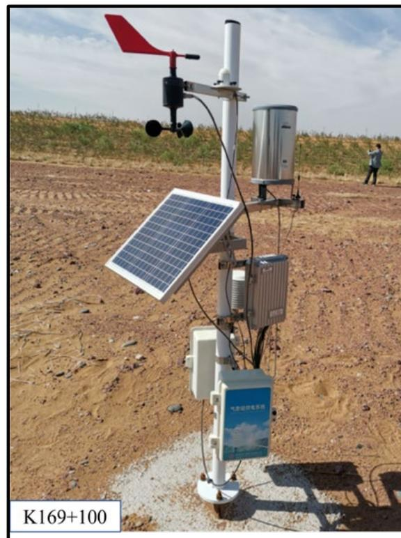
**Figure 2.** Remote Weather Monitoring Station.
