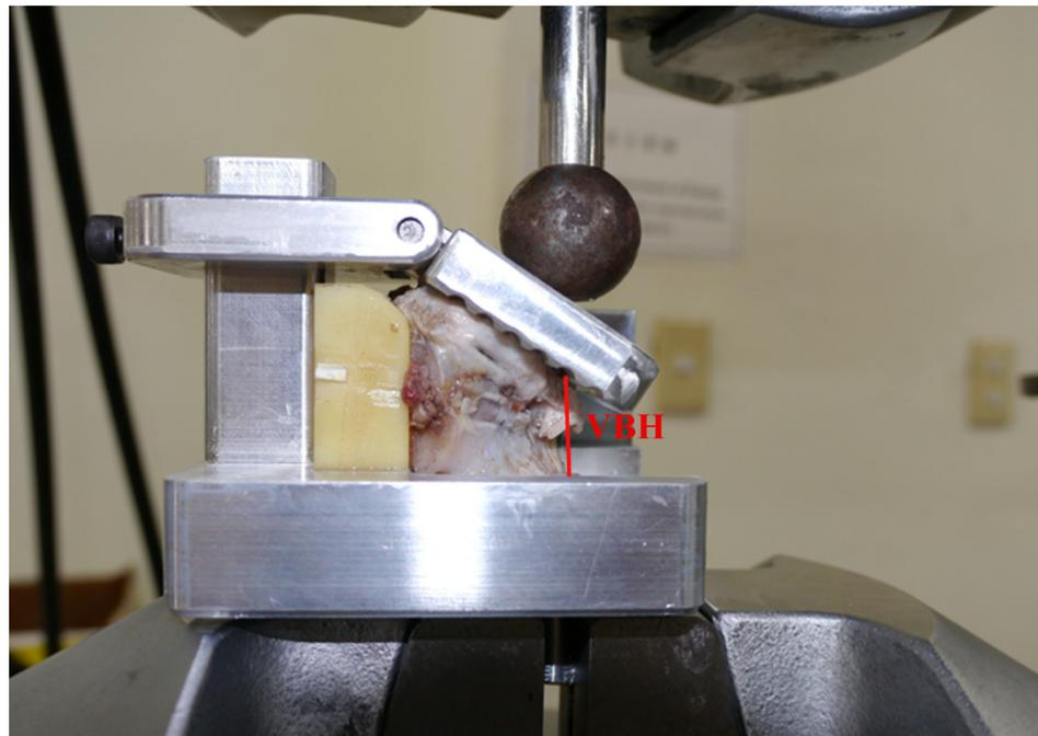
**Figure 1.** Photograph showing the experimental setup of the compression test. The main vector of the axial force was centered at the end plate of the anterior fourth of the vertebral body to create wedge compression of the anterior vertebral body.
