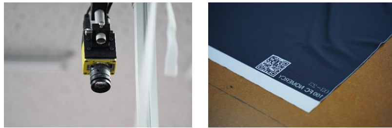
Figure 16. Order information recognition using vision system in the cutting process.
