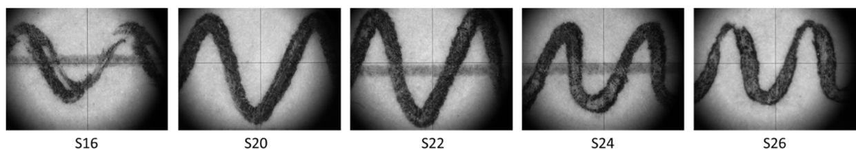
Figure 13. Lines drawn at different motor speeds as viewed through the microscope.
