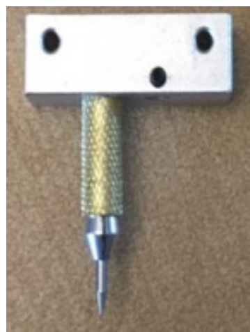
Figure 3. The adapter used for attaching the pen to the cartridge.
