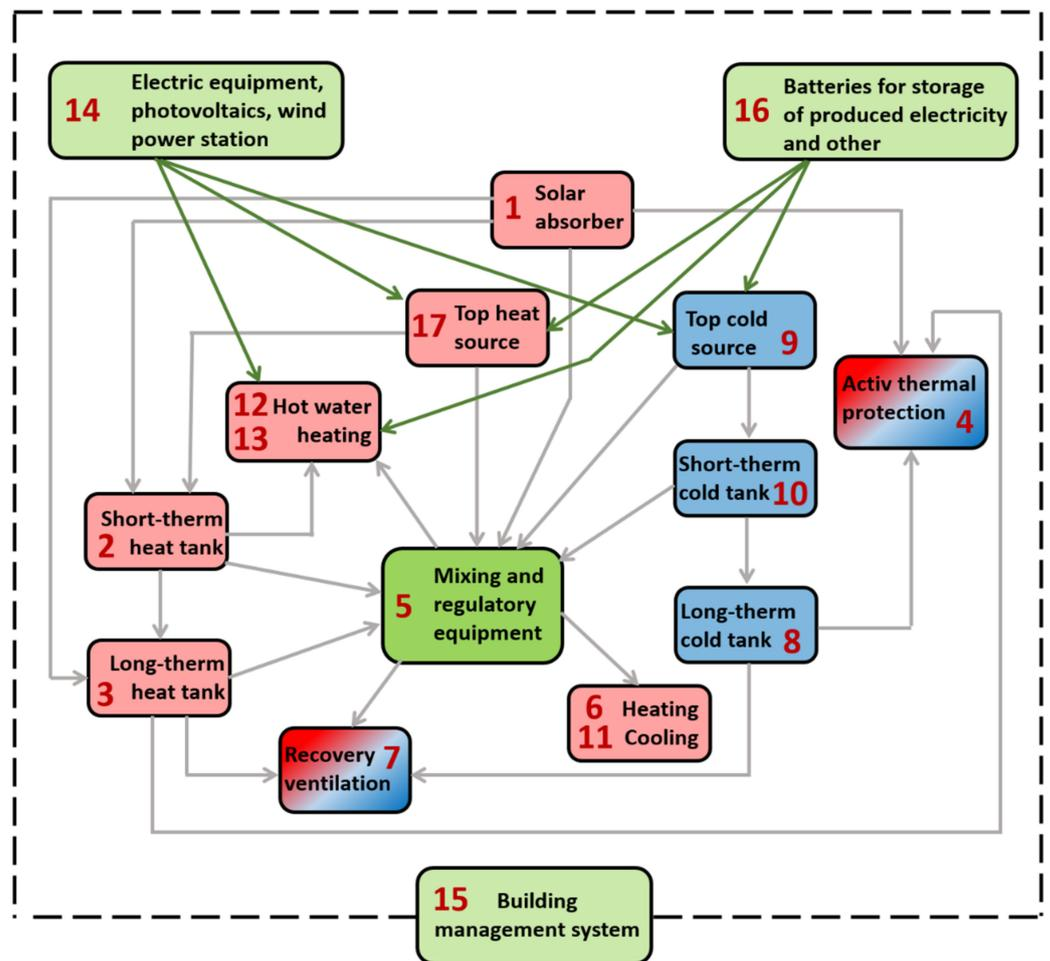
**Figure 6.** Variants of power equipment cooperate in different modes of operation.
