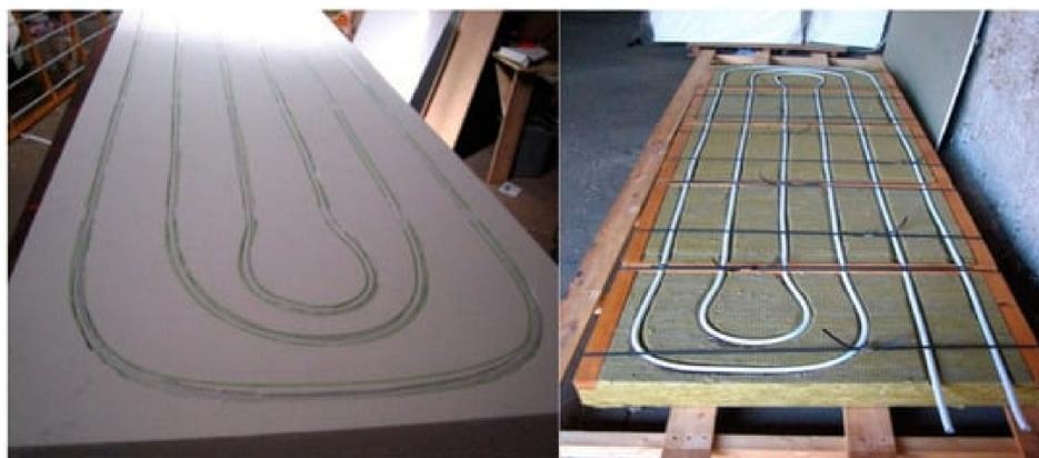
**Figure 14.** View of prototypes of insulation panels with integrated active thermal protection, on the left made of polystyrene, on the right of mineral wool. [Author: Kalús].
