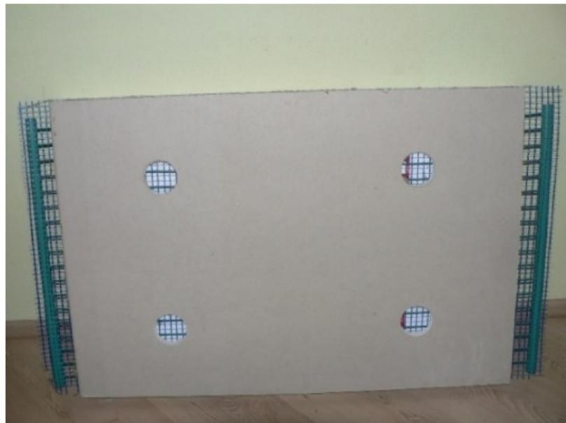
**Figure 16.** View of a prototype interior panel with capillary mat application for heating/cooling. [Author: Kalús].
