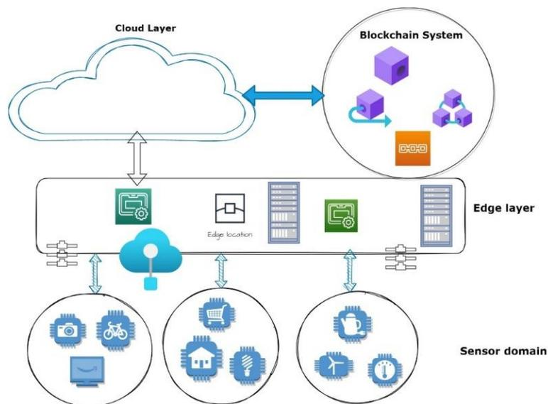
**Figure 1.** The proposed Blockchain-enabled IoT System’s architecture.
