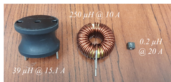
Figure 18. Comparison between two energy storage inductors and a tiny resonant inductor.
