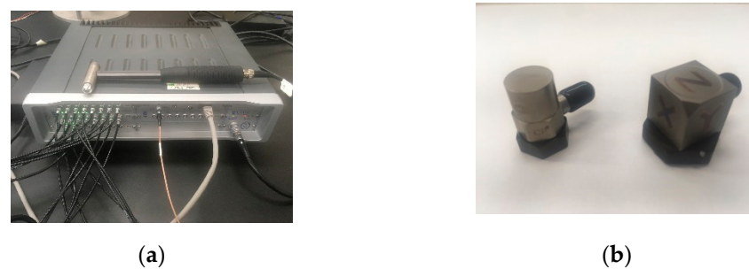
Figure 4. Equipment for the impact hammer test: (a) digital acquisition (DAQ) system and impact hammer; (b) single-axial (left), and tri-axial (right) accelerometer.
