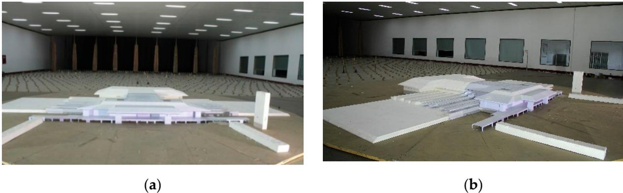
**Figure 2.** Wind tunnel test for rigid model pressure measurement: (a) front view; (b) side view.
