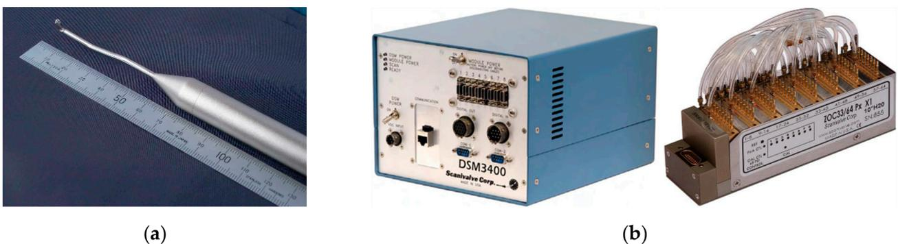
**Figure 1.** Test data acquisition device: (a) TFI Cobra three-dimensional fluctuating anemometer; (b) Scanivalve DSM4000 electronic pressure scanning valve system.
