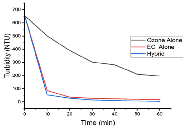
**Figure 3.** Turbidity reduction for separate processes such as pure ozone, electrocoagulation and coupled process of EC/O<sub>3</sub>, operated at conditions of 10.0 volts, feed flow 360 L/h, O<sub>3</sub> flow 2400 mg/h, pH 6.89, and initial turbidity of 655 NTU.
