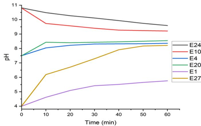
Figure 4. Variation of the pH in the time of treatment by electrocoagulation/O<sub>3</sub>.
