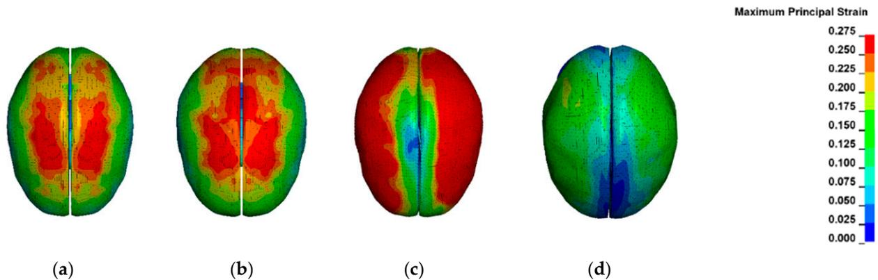
**Figure 10.** Maximum principal strain on the brain obtained from the inclined drop tests at (a) crown, (b) front, (c) rear, and (d) side locations.
