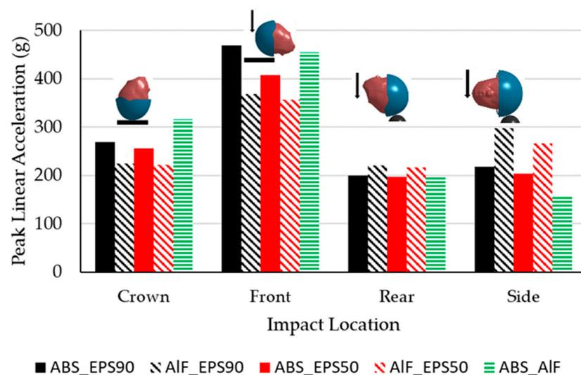
**Figure 11.** Comparisons of the peak linear acceleration obtained from the DOT drop test for five combinations of helmet material.
