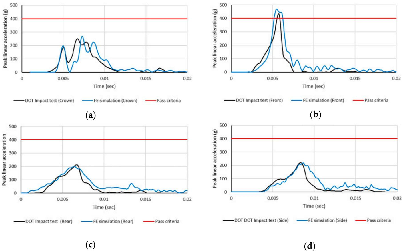
**Figure 7.** Comparisons of the linear acceleration obtained from the DOT drop test and the finite element simulations at (a) crown, (b) front, (c) rear, and (d) side impact locations.
