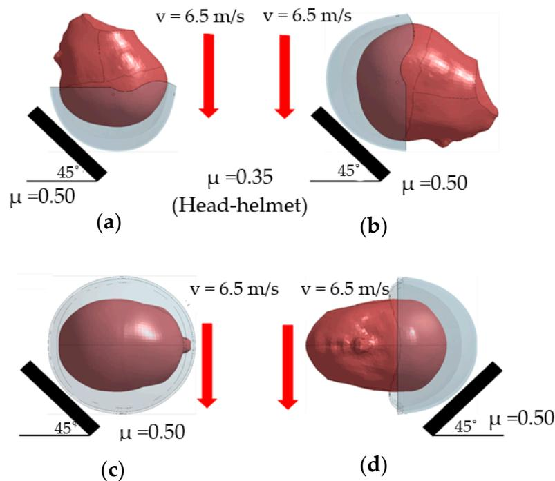
**Figure 4.** Model setup for the 45° inclined drop test at (a) crown, (b) front, (c) rear, and (d) side.
