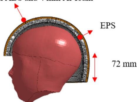
**Figure 5.** The modified child helmet with uniform liner thickness.
