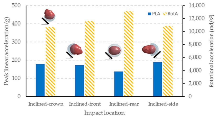
**Figure 9.** The peak linear (PLA) and the rotational accelerations (RotA) obtained from the inclined drop tests at four impact locations.
