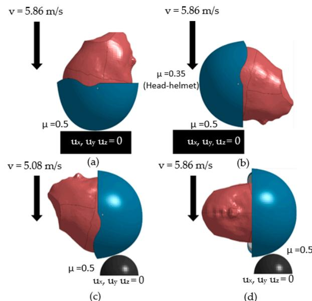
**Figure 3.** Model setup for the DOT drop test at (a) crown, (b) front, (c) rear, and (d) side locations.
