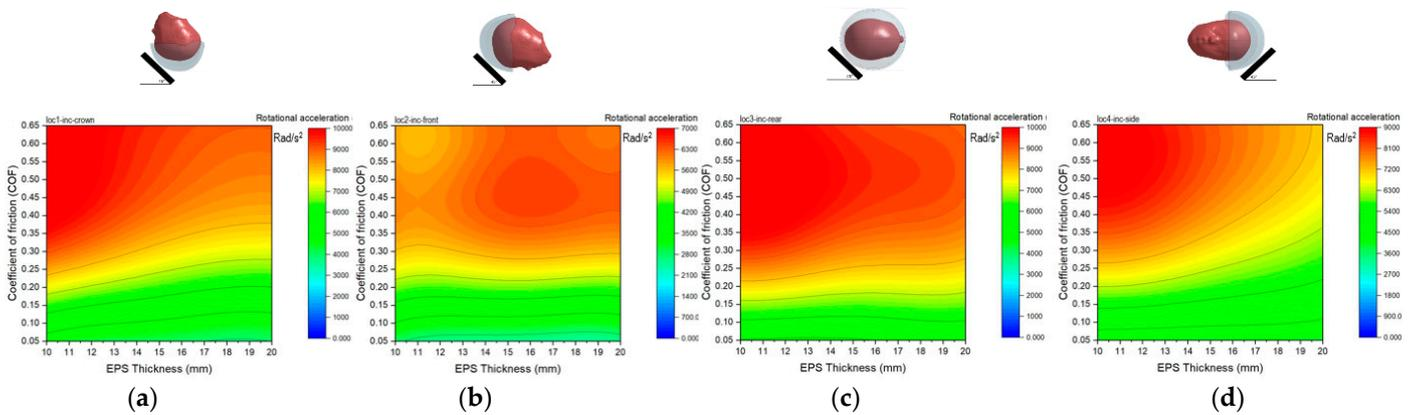
**Figure 15.** Relationship between helmet parameters and the rotational acceleration predicted by the ROM with the inclined anvil drop test at (a) crown, (b) front, (c) rear, and (d) side impact locations.
