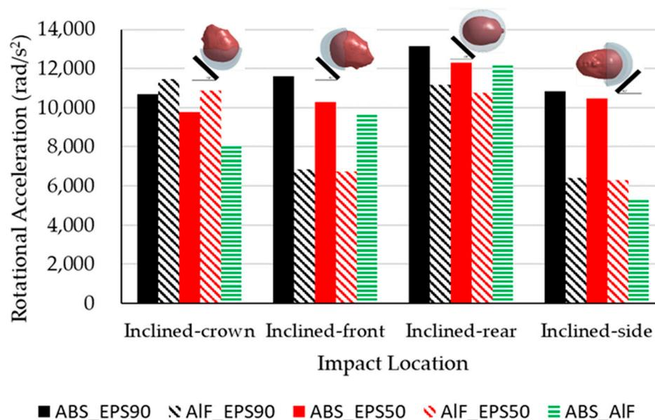
**Figure 12.** Comparisons of the peak rotational acceleration obtained from the inclined anvil drop test for five combinations of helmet material.
