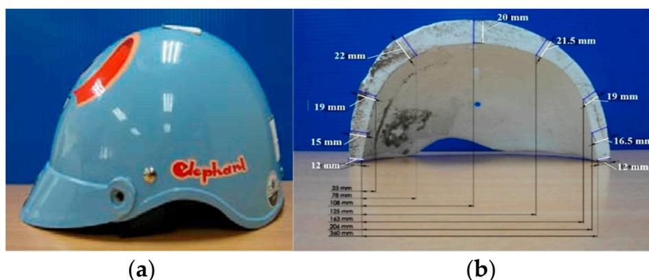
**Figure 1.** (a) A child motorcycle helmet sold in Thailand (b) the half section of the inner liner.
