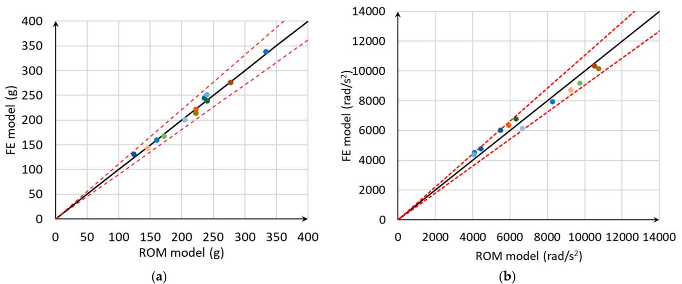
**Figure 13.** Scatter plots of prediction errors for both a peak (a) linear acceleration and a (b) rotational acceleration.
