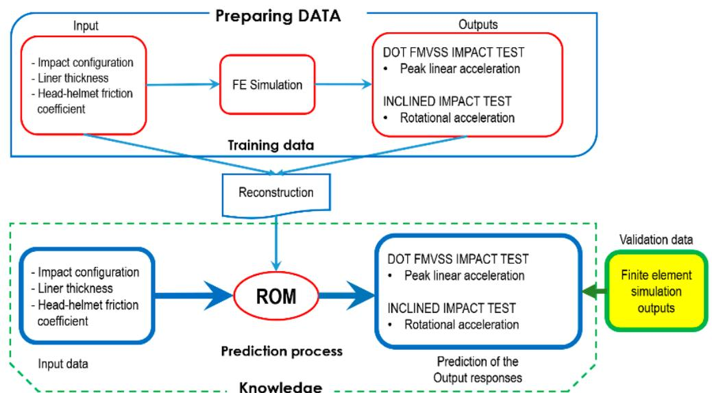
**Figure 6.** Reduced-order model establishment process.
