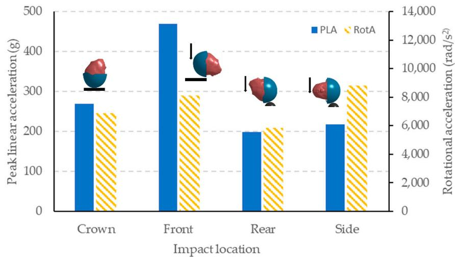
**Figure 8.** The peak linear (PLA) and the rotational accelerations (RotA) obtained from the DOT drop tests at four impact locations.
