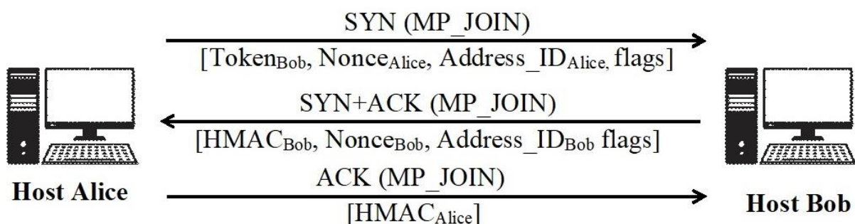
Figure 4. MPTCP Options in Version (v0) adding new subflow using MP_JOIN.
