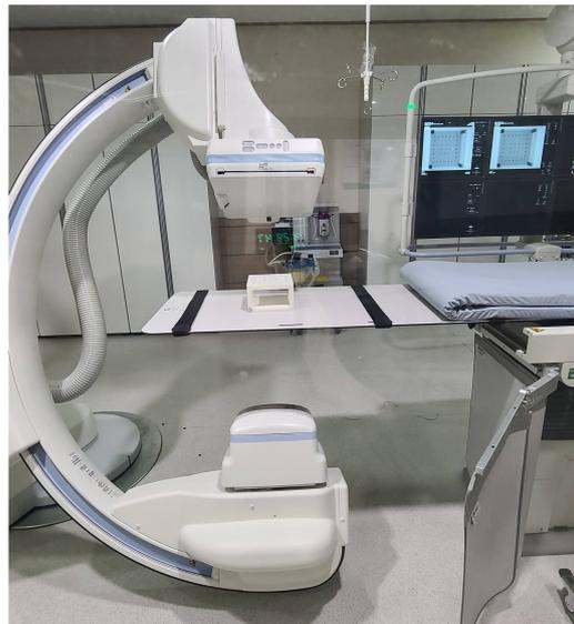
**Figure 6.** C-arm angio imaging device was applied to the experiment, which has the functions of 2D projectional X-ray imaging and CBCT imaging.
