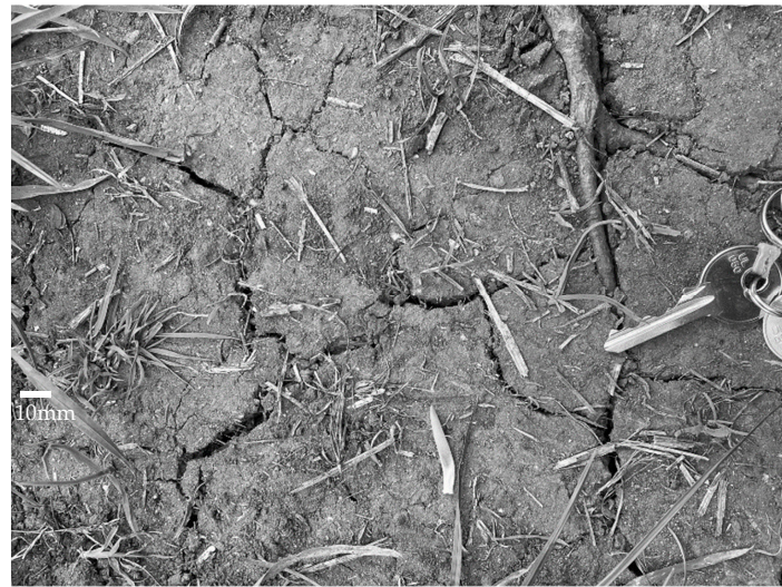
Figure 14. Example of desiccation cracks observed in Baile Hill (York) heritage asset.
