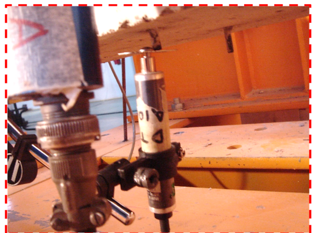
Figure 3. (a) Experimental setup and instrumentation of the full-scale beam-column joint specimens under lateral imposed cyclic reversal deformations; and (b) LVDT set for measuring the slip of the beams' longitudinal CFRP bars (two LVDTs with 0.01 mm accuracy).
