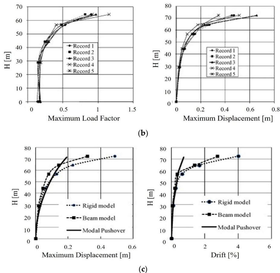
**Figure 8.** Seismic assessment of the Qutb Minar tower. Comparison of the results from different analysis methods [64]: (a) capacity curves for pushover analyses, (b) maximum load factor and displacements along the minaret height for dynamic analyses, (c) displacements and drifts along the minaret height for modal pushover and non-linear dynamic analyses.
