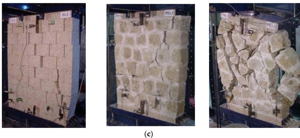
**Figure 3.** Experimental results on stone masonry shear walls [21]: (a) specimen geometries; (b) force–displacement diagrams; (c) failure mechanisms.
