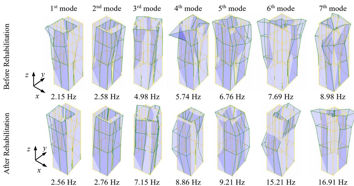
**Figure 6.** Experimental mode shapes of the Mogadouro clock tower—undeformed structure in yellow wireframe (reprinted with permission from Ref. [49]. Copyright 2018, Elsevier).
