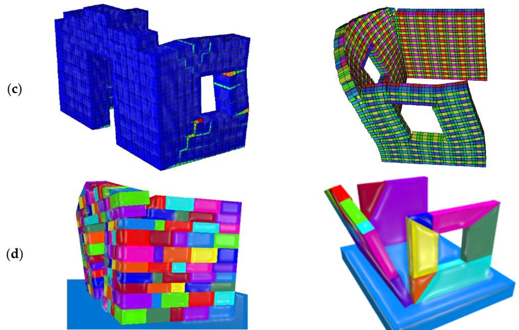
**Figure 11.** Examples of models adopted for the blind predictions of the (a) tested masonry structures: (b) models with rigid macro-blocks; (c) FEM models and (d) DEM models.
