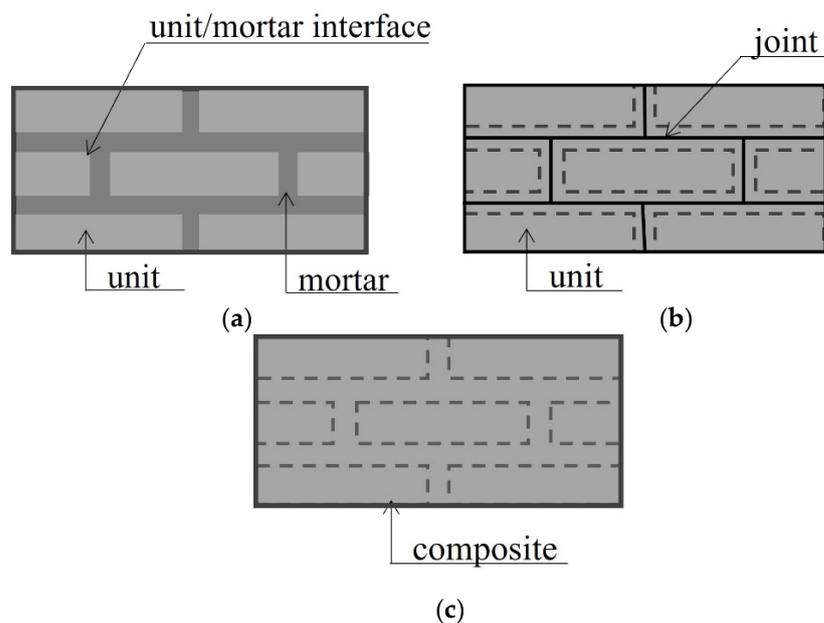
**Figure 10.** Modelling strategies for masonry structures (adapted from [27]): (a) detailed micro-modelling, (b) simplified micro-modelling, (c) macro-modelling.
