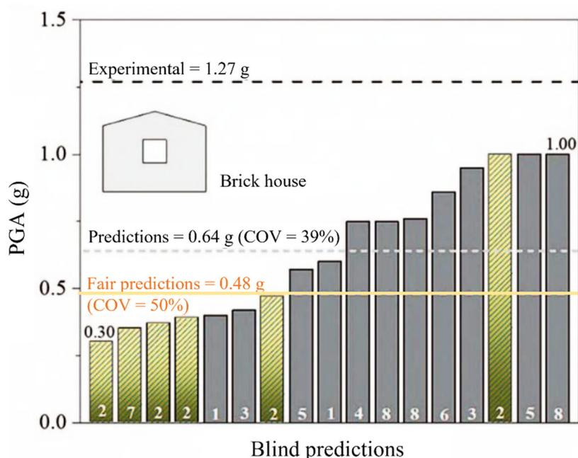
**Figure 12.** Seismic acceleration capacity (PGA) obtained from the blind predictions [98] (green and yellow bars correspond to good and fair mechanism predictions).
