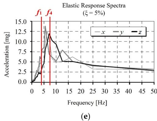
**Figure 4.** Seismic response of the Church of Jerónimos Monastery, Portugal (adapted from [46,47]): (a) exterior view; (b) location of strong motion recorders (A1: chancel base; A2: nave vault extrados); (c,d) acceleration response at the base and at the top of the nave during the earthquake; (e) measured response spectra.
