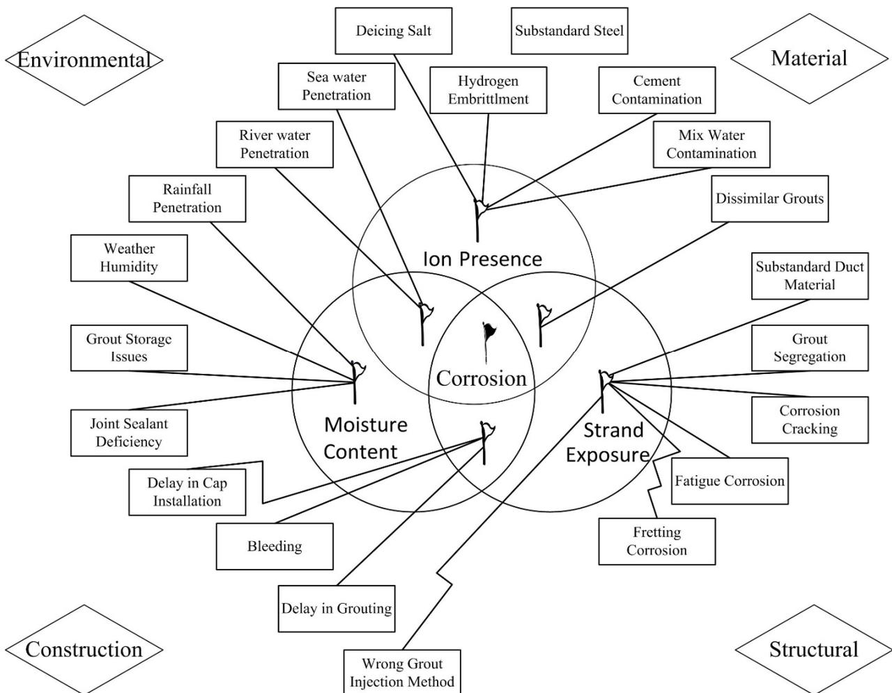
Figure 2. Classification of factors involved in corrosion of external post-tensioning system.
