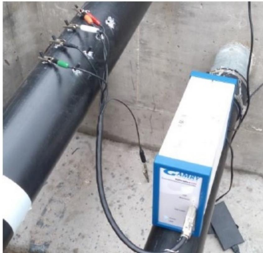
**Figure 6.** Electrochemical impedance spectrometer [9].
