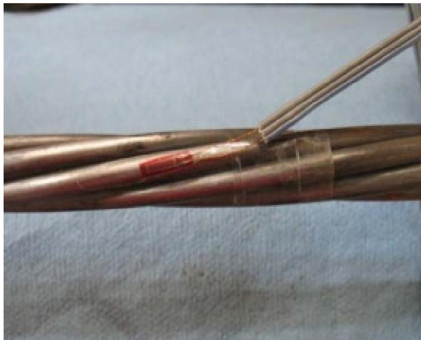
**Figure 10.** Strain gauge on the post-tensioning strand [9].
