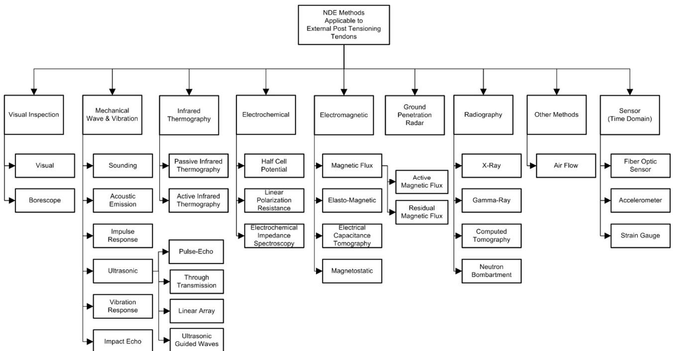
Figure 3. Classification of NDE methods applicable to external post-tensioning system.
