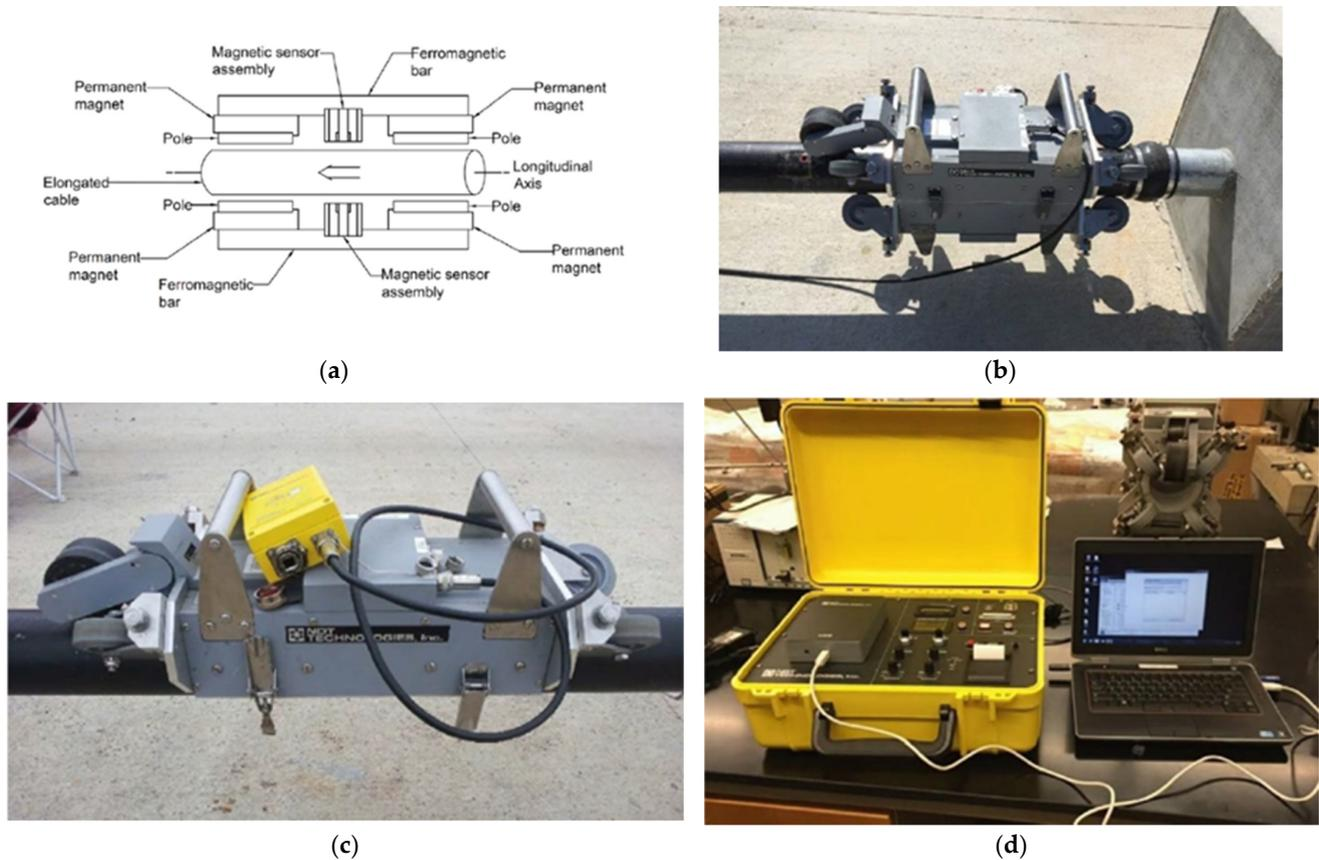
**Figure 7.** Magnetic flux leakage (a) sensor probe, (b) full head sensor, (c) half head sensor, (d) the connection of the NDE extension to the computer [9].
