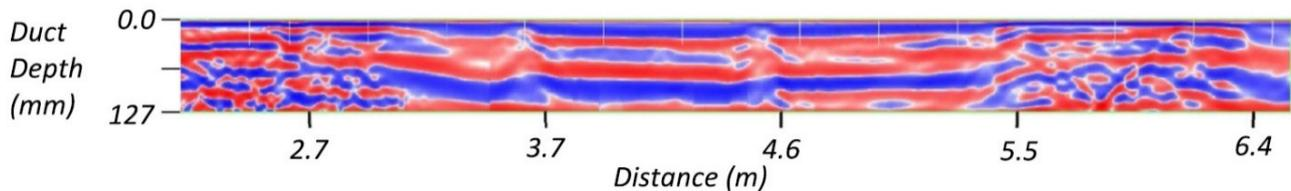
**Figure 8.** Photo captured by ground penetration radar [9].
