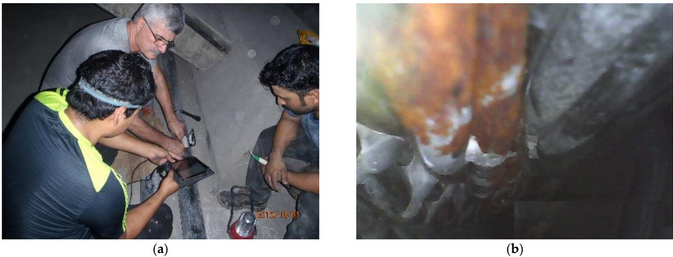
**Figure 15.** Activities during the second stage of two-stage inspection. (a) application of video-borescope, (b) a sample of steel photo captured by borescope.
