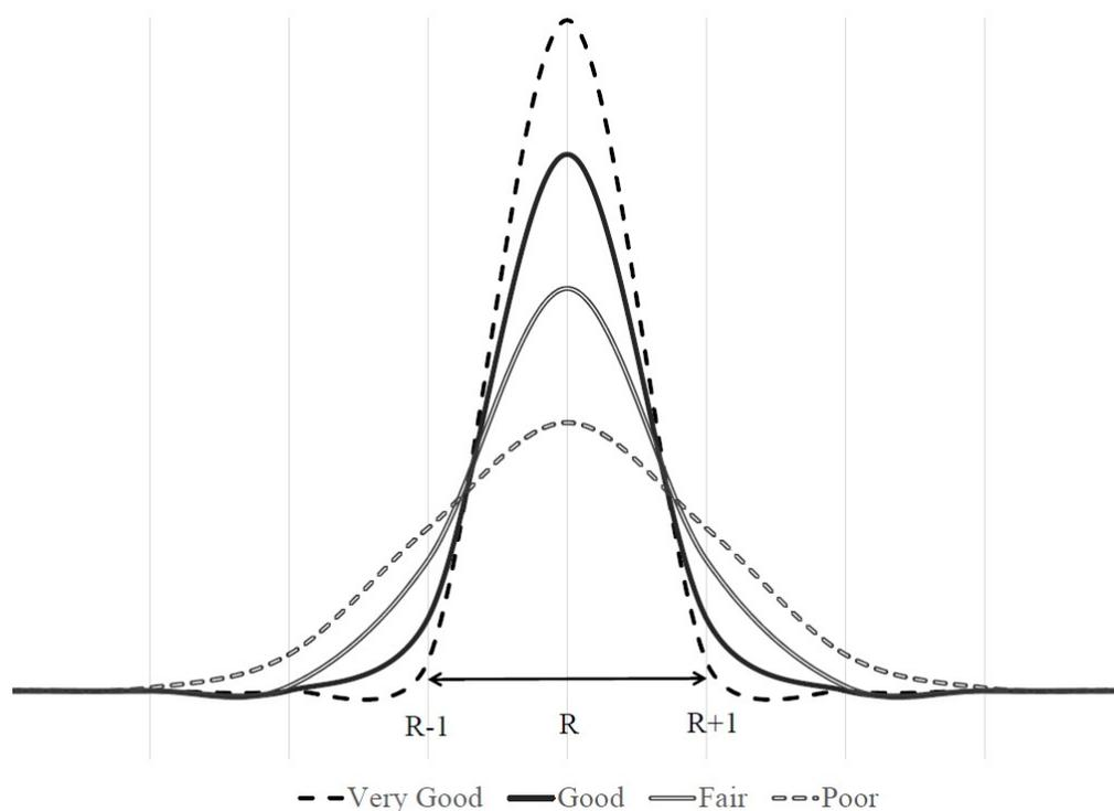
**Figure 11.** Accuracy Levels of NDE methods.
