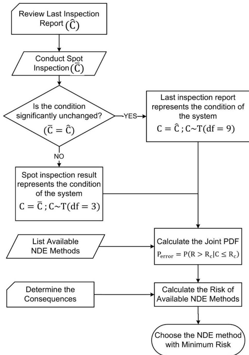
**Figure 1.** General procedure for risk-based selection of inspection method.
