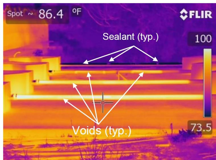
**Figure 5.** Photo captured by infrared thermography with interpretation [9].
