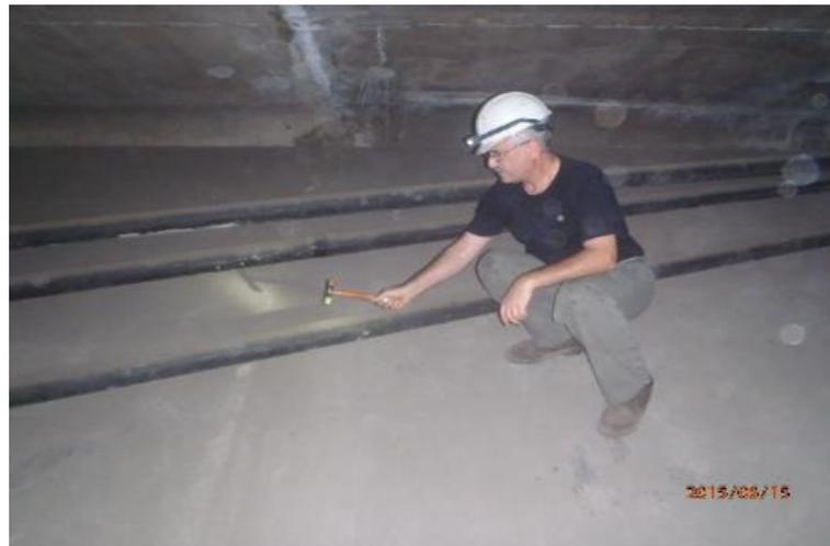
**Figure 4.** Sounding used for spot inspection.
